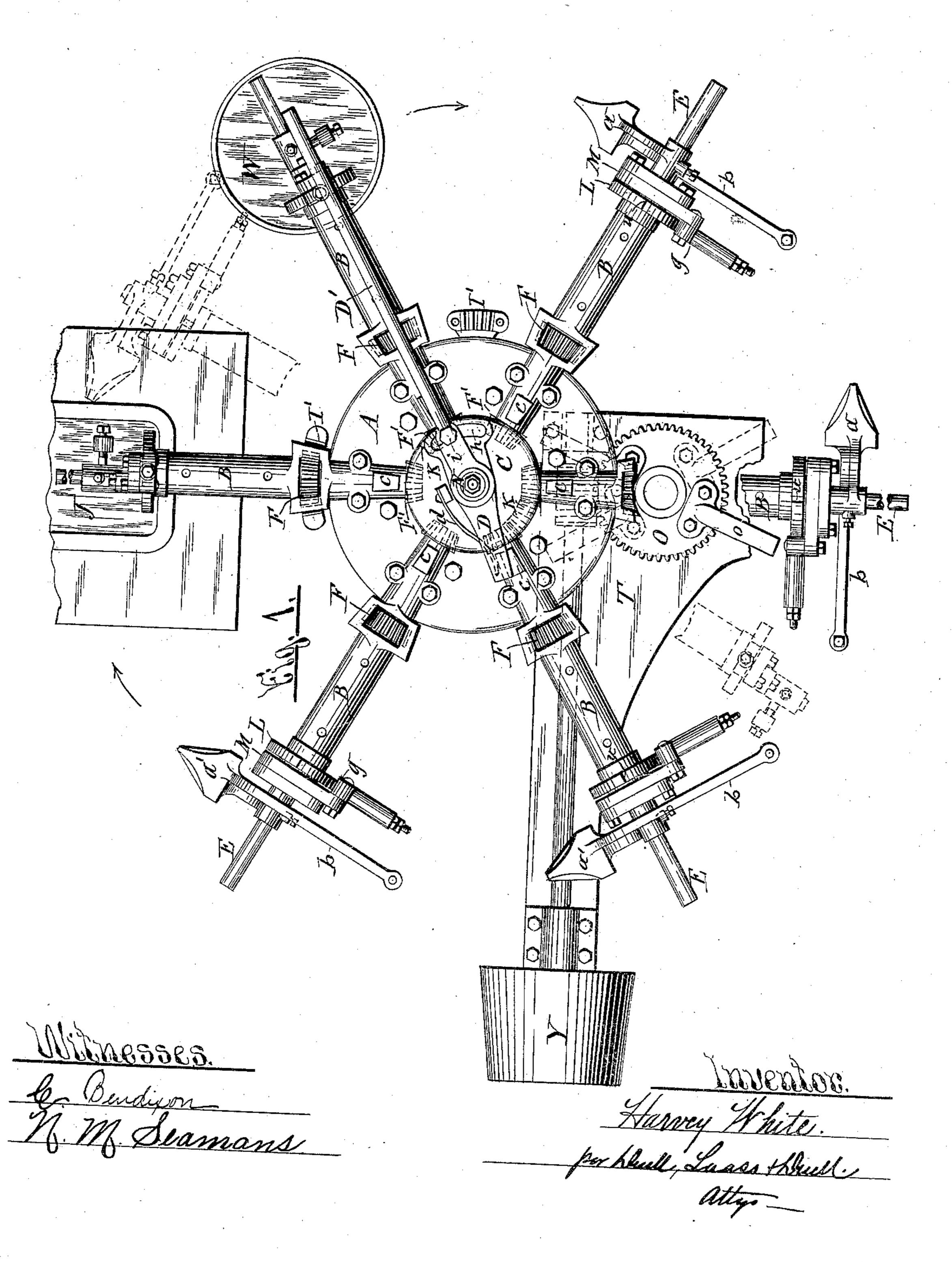
MACHINE FOR HEATING AND HARDENING METAL ARTICLES.
