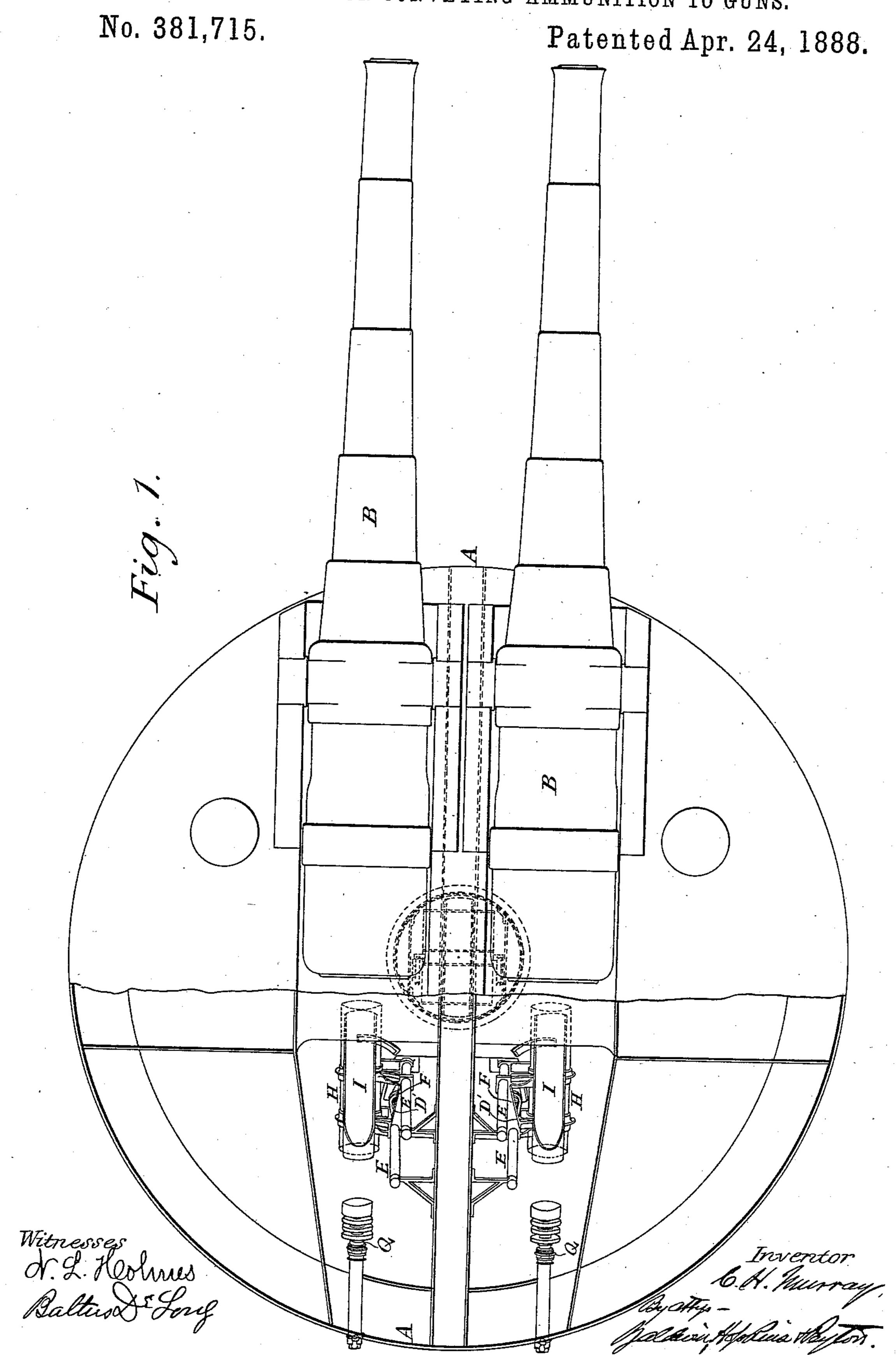
APPARATUS FOR CONVEYING AMMUNITION TO GUNS.
