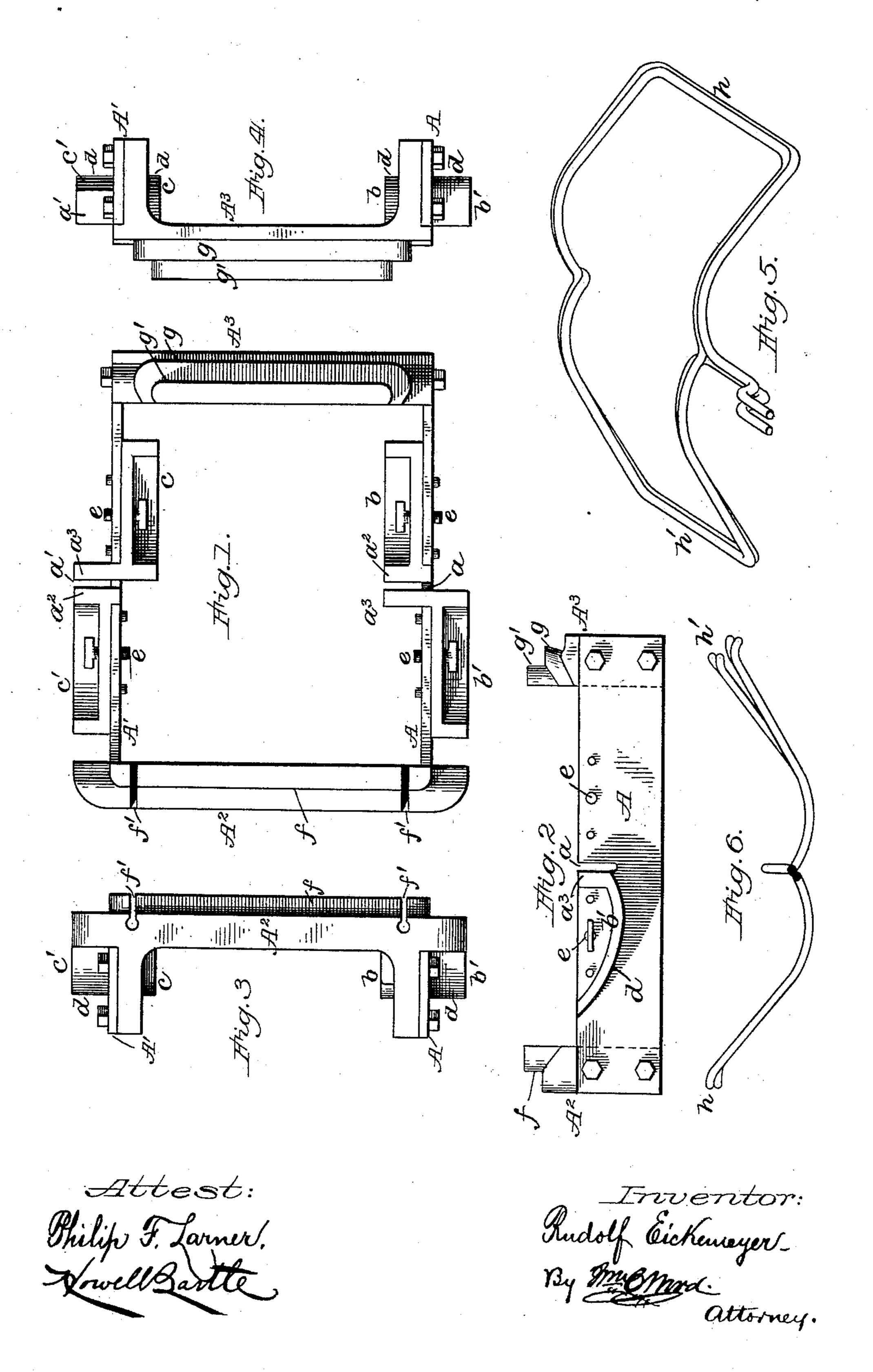
FRAME FOR WINDING ARMATURE COILS.
