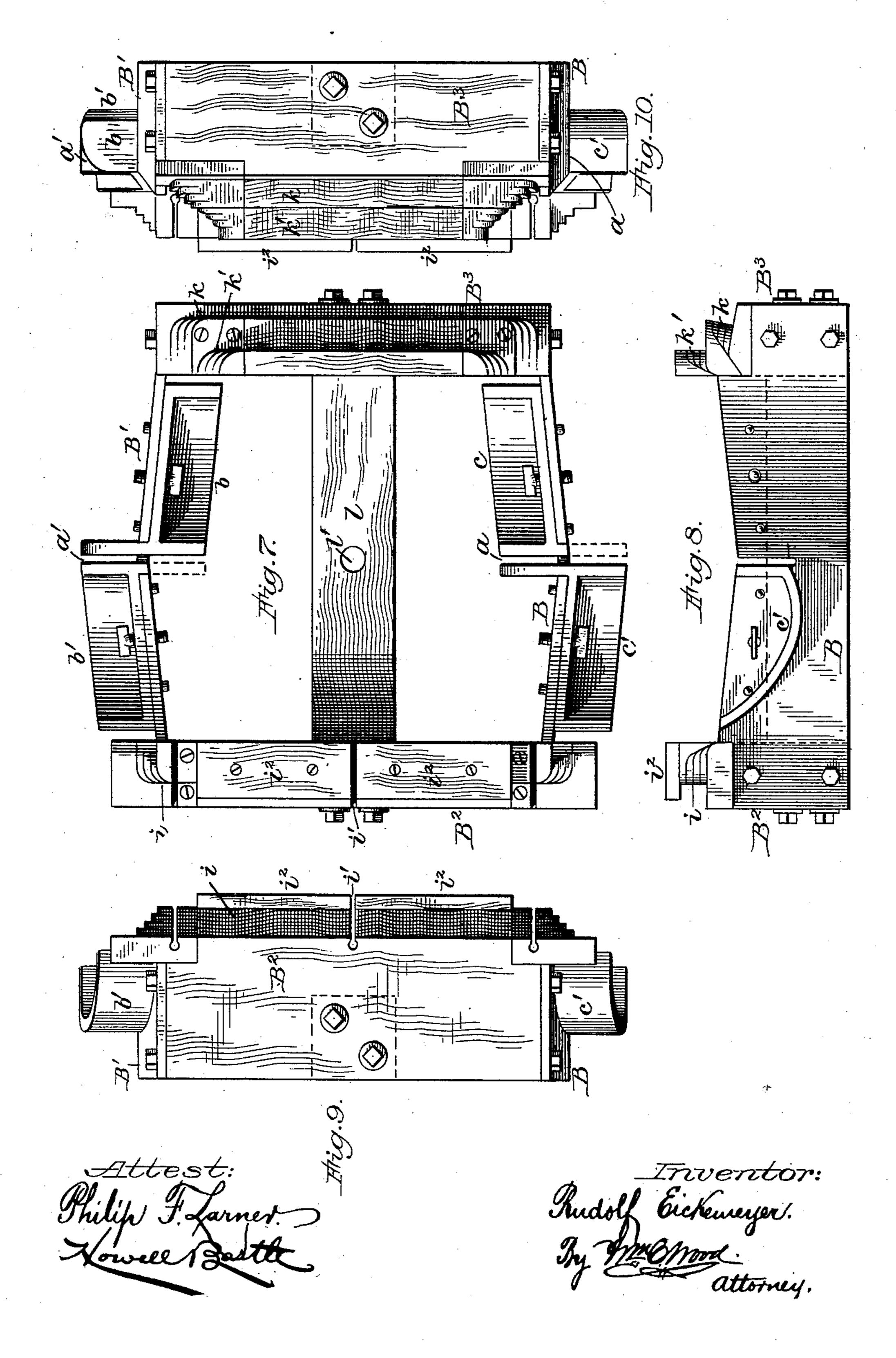
FRAME FOR WINDING ARMATURE COILS.
