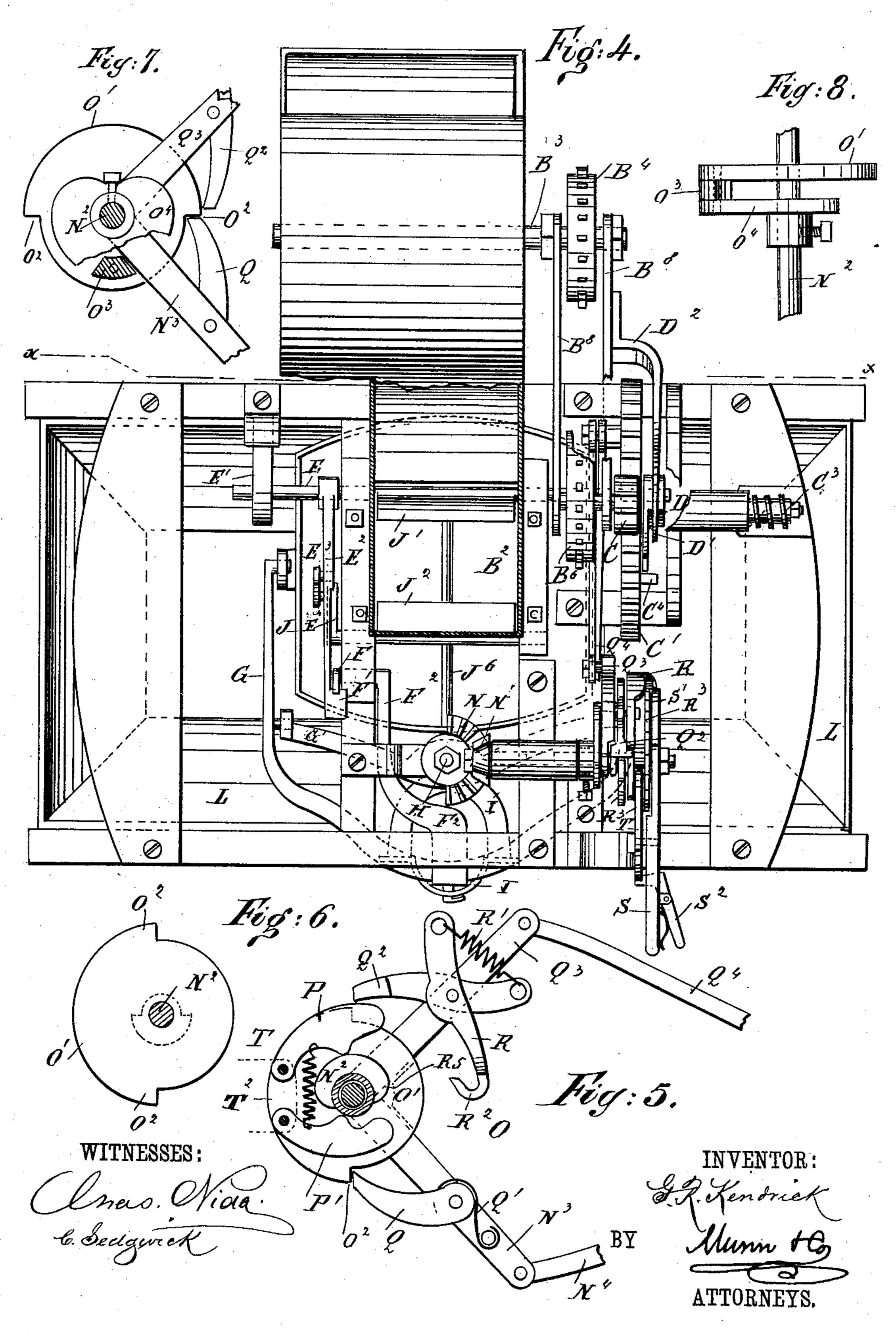
GRAIN WEIGHING, REGISTERING, AND BAGGING MACHINE.
