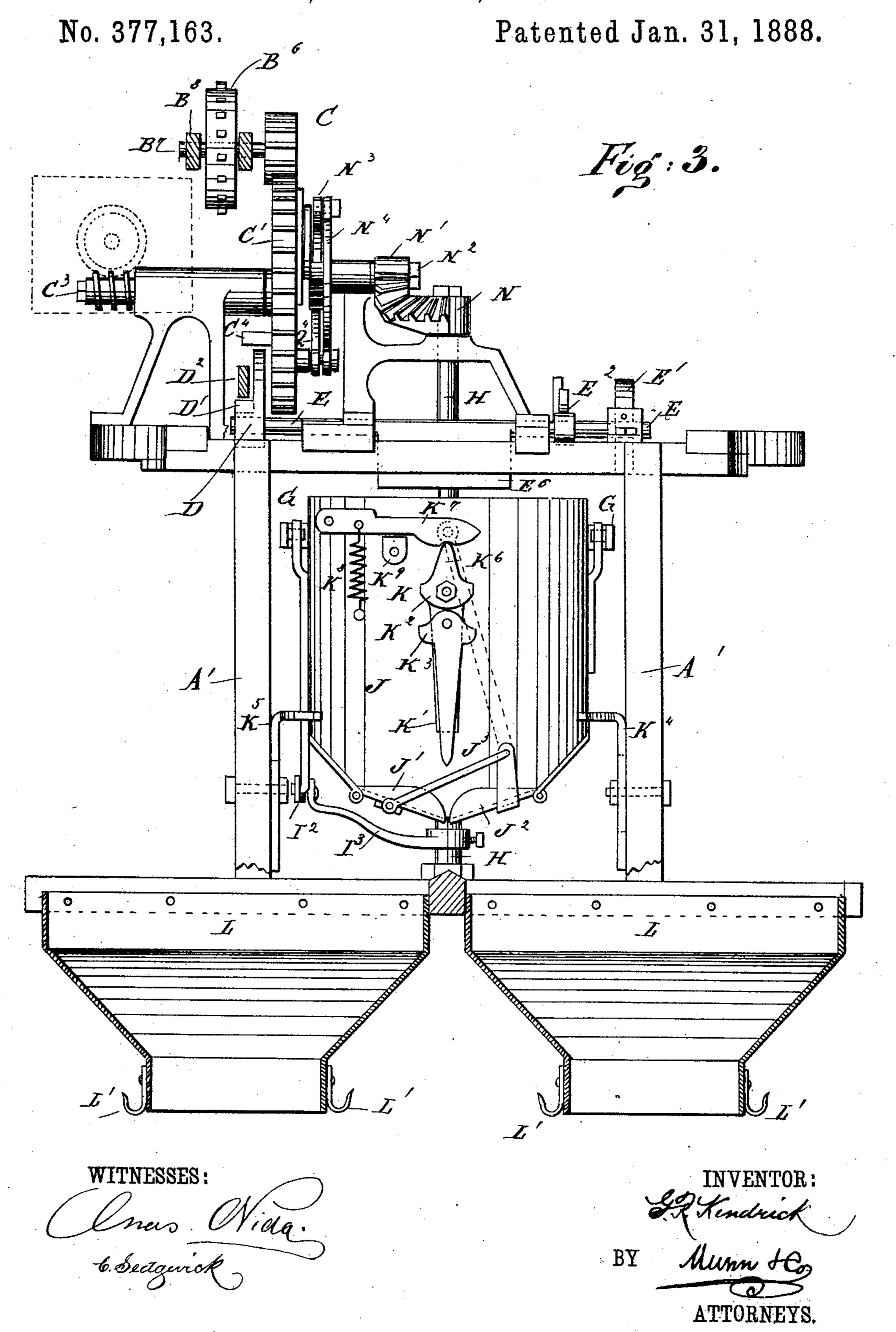
GRAIN WEIGHING, REGISTERING, AND BAGGING MACHINE.
