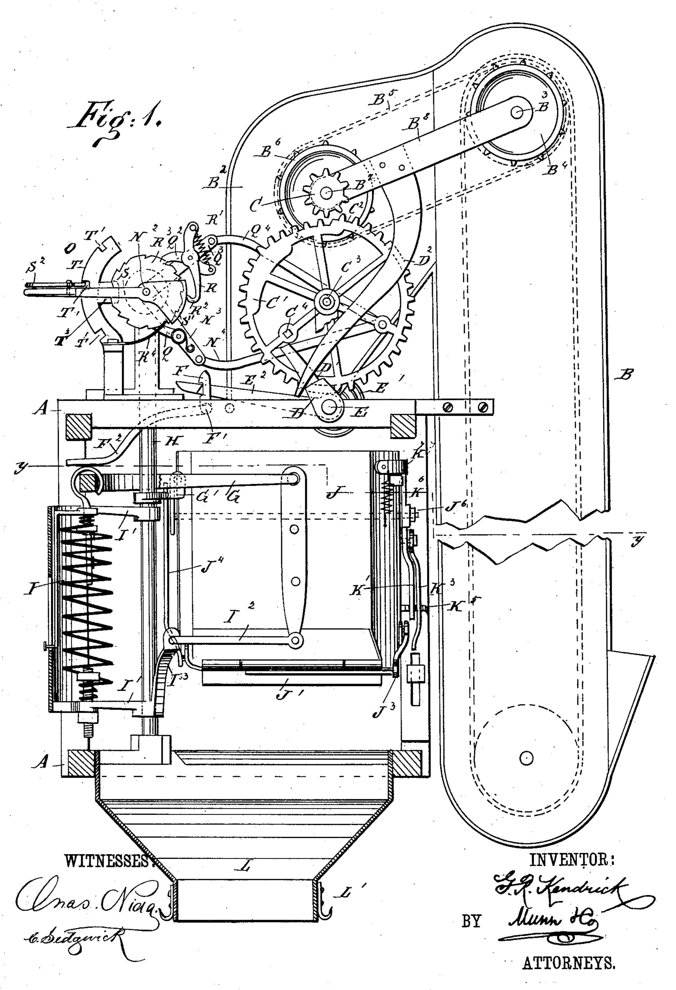
GRAIN WEIGHING, REGISTERING, AND BAGGING MACHINE.
