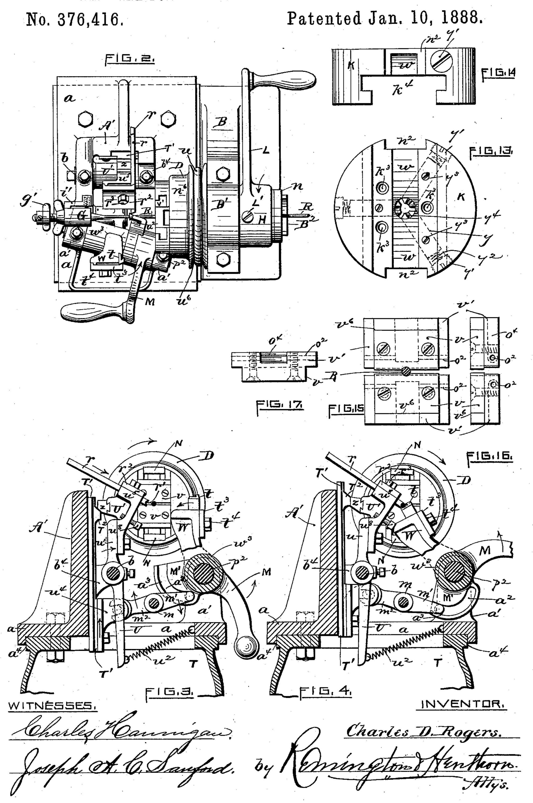
MACHINE FOR FINISHING HEADS OF SCREW BOLTS.
