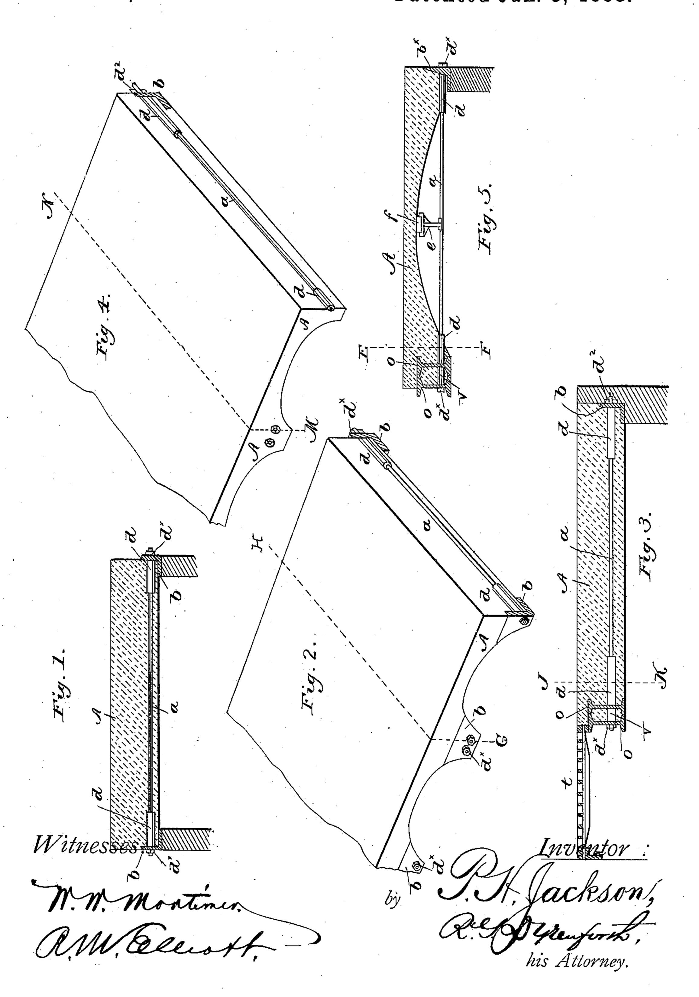
CONSTRUCTION OF ARTIFICIAL STONE OR CONCRETE PAVEMENTS.
