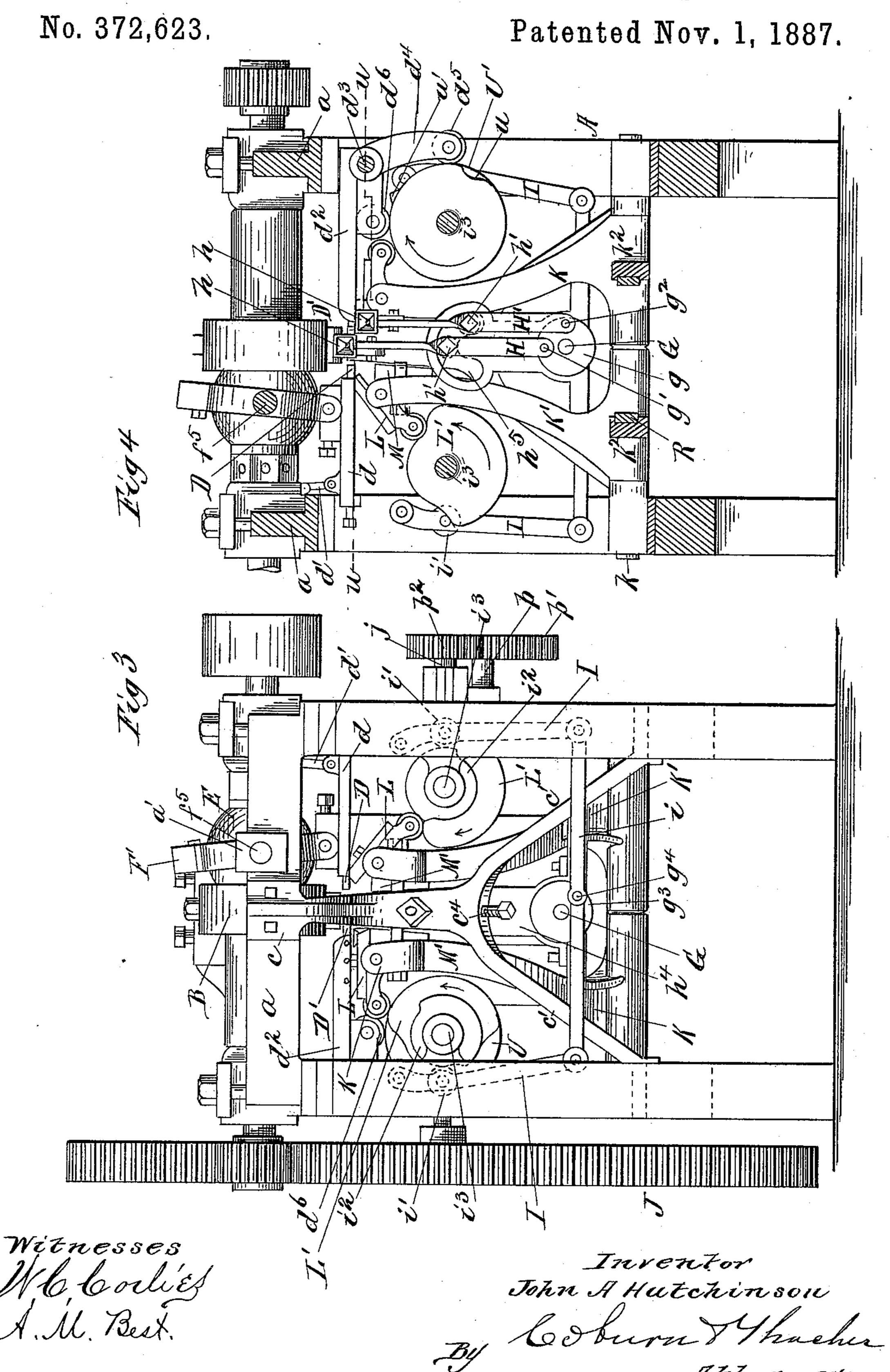
MACHINE FOR FORGING HORSESHOE NAILS.
