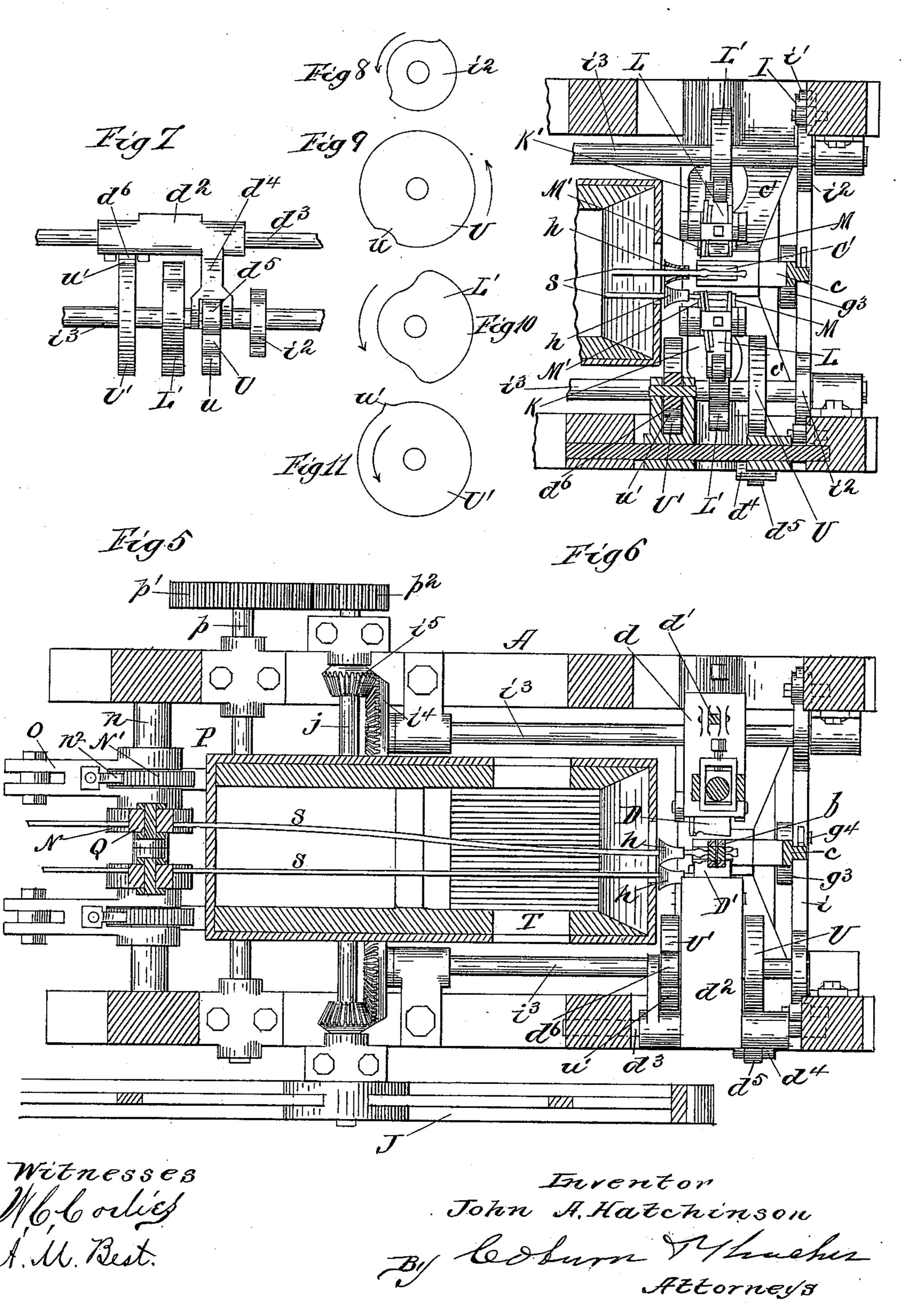
MACHINE FOR FORGING HORSESHOE NAILS.
