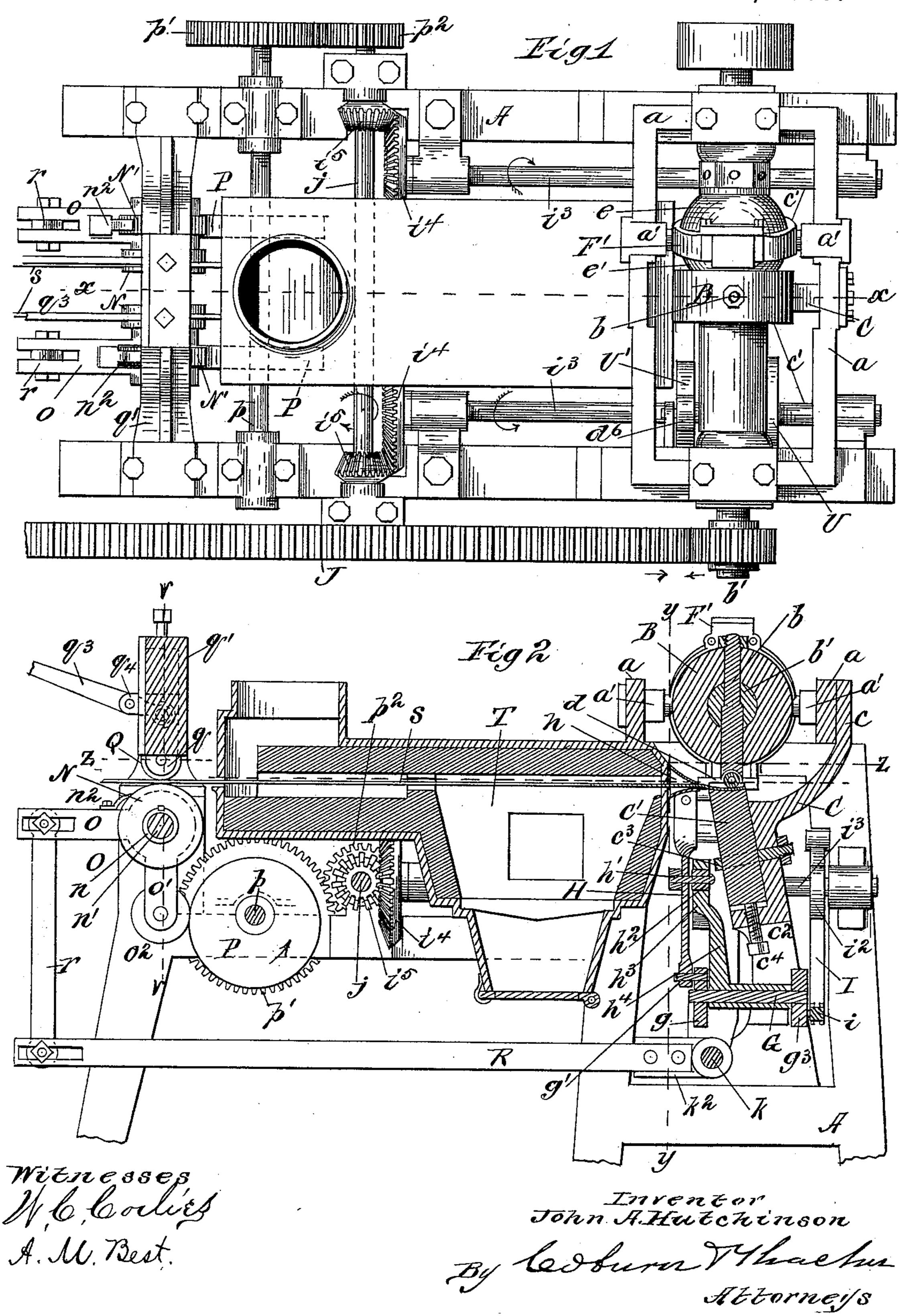
MACHINE FOR FORGING HORSESHOE NAILS.
