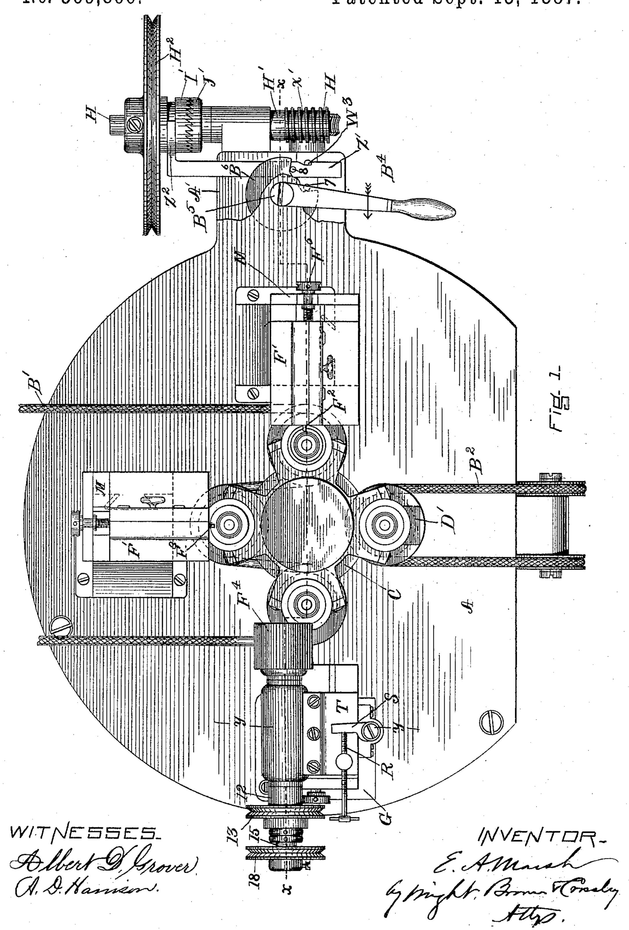
MACHINE FOR TURNING AND POLISHING THE RIMS OF WATCH BALANCES.
