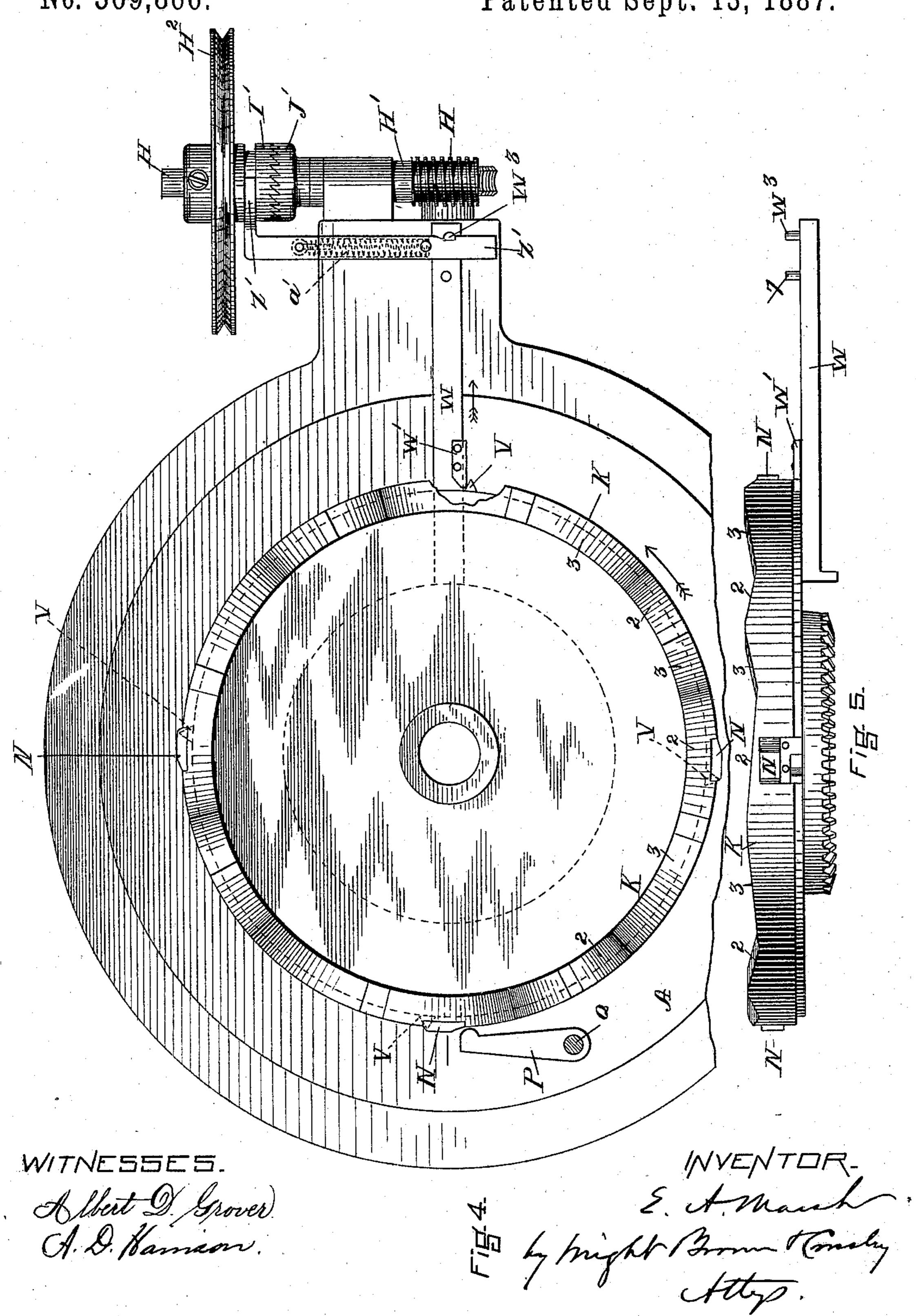
MACHINE FOR TURNING AND POLISHING THE RIMS OF WATCH BALANCES.
