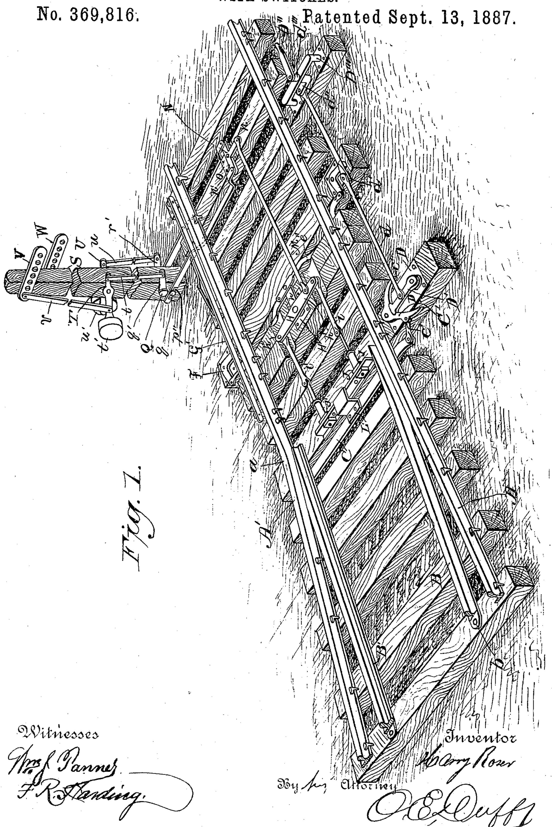
MEANS FOR OPERATING RAILWAY DANGER SIGNALS IN CONNECTION WITH SWITCHES.
