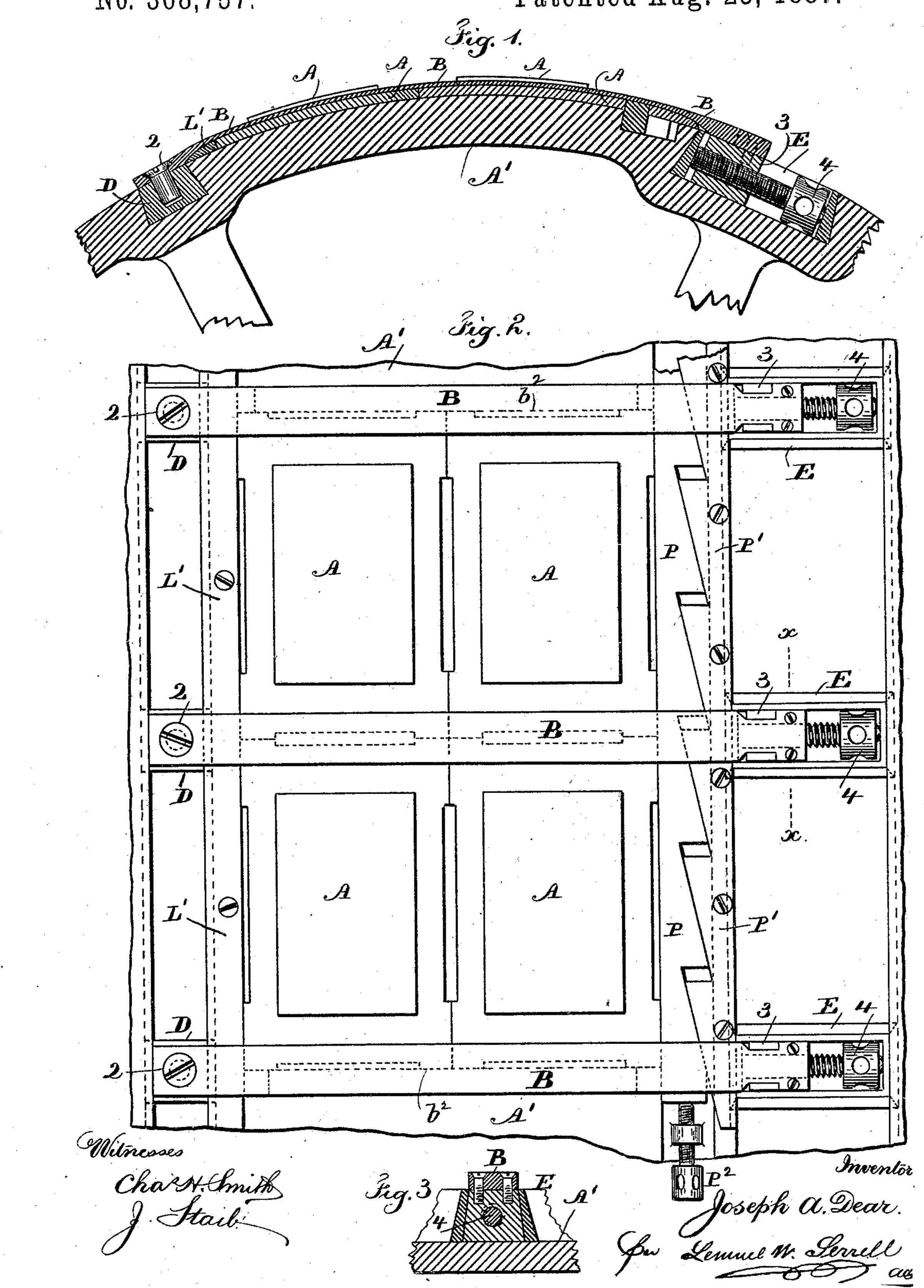
FASTENING FOR PRINTING PLATES UPON CYLINDRICAL SURFACES.
