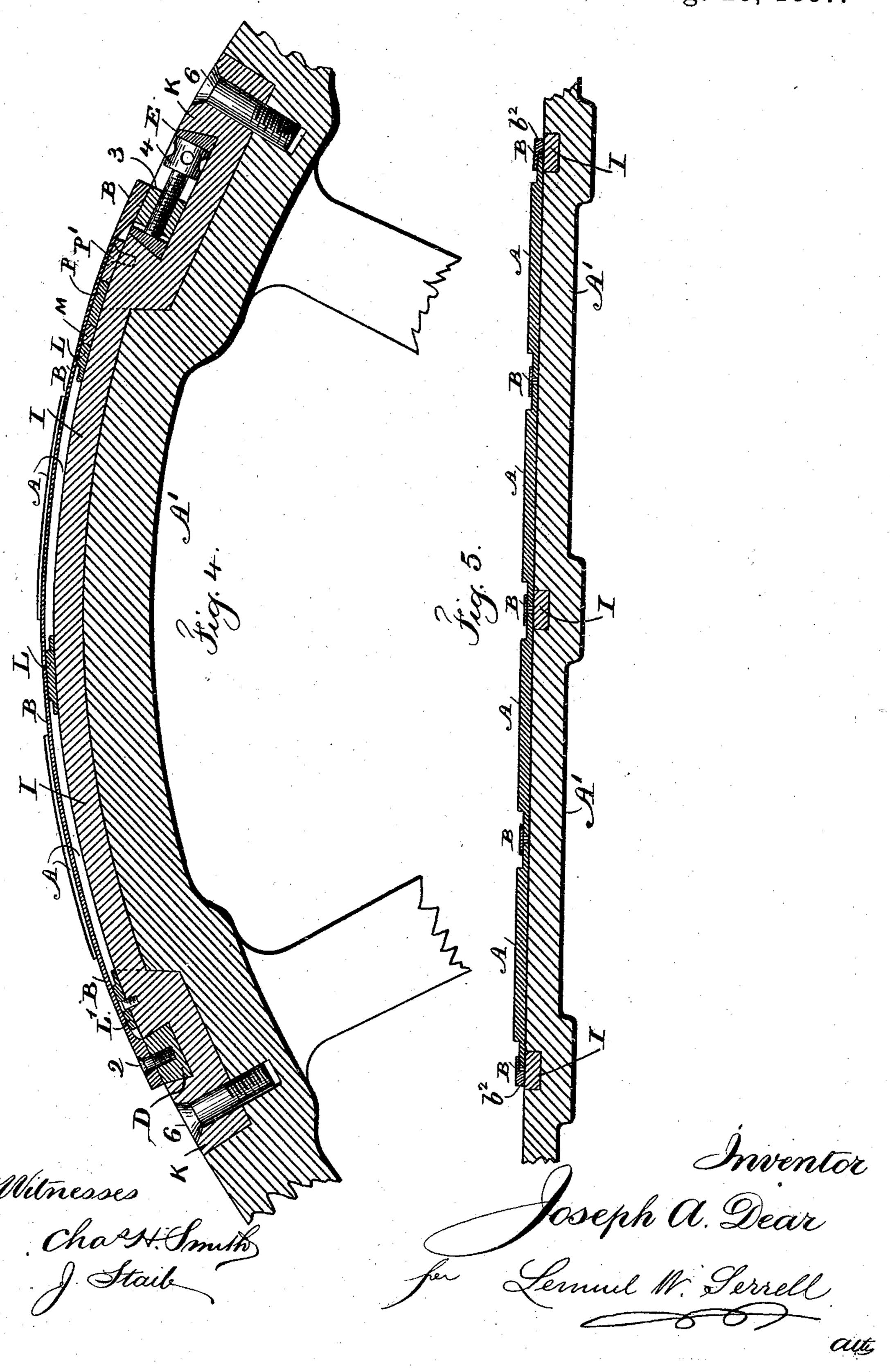
FASTENING FOR PRINTING PLATES UPON CYLINDRICAL SURFACES. No. 368,757. Patented Aug. 23, 1887.
