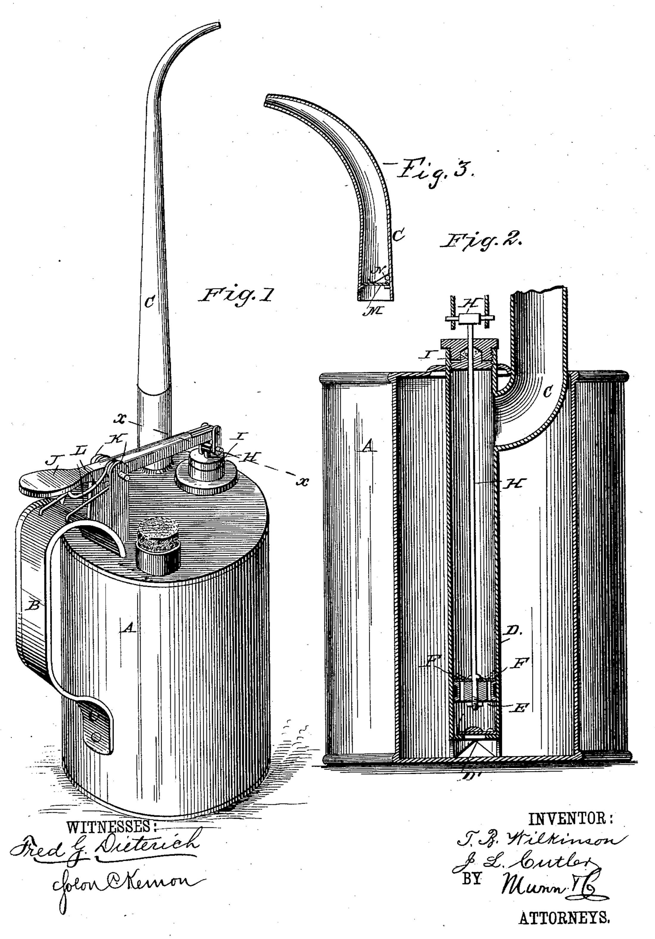
raised the pressure of the oil opens this valve to allow the oil to be thrown out of the spout, and as soon as this pressure is removed by the piston being lowered the spring N closes the valve M automatically and cuts off further flow of oil.
