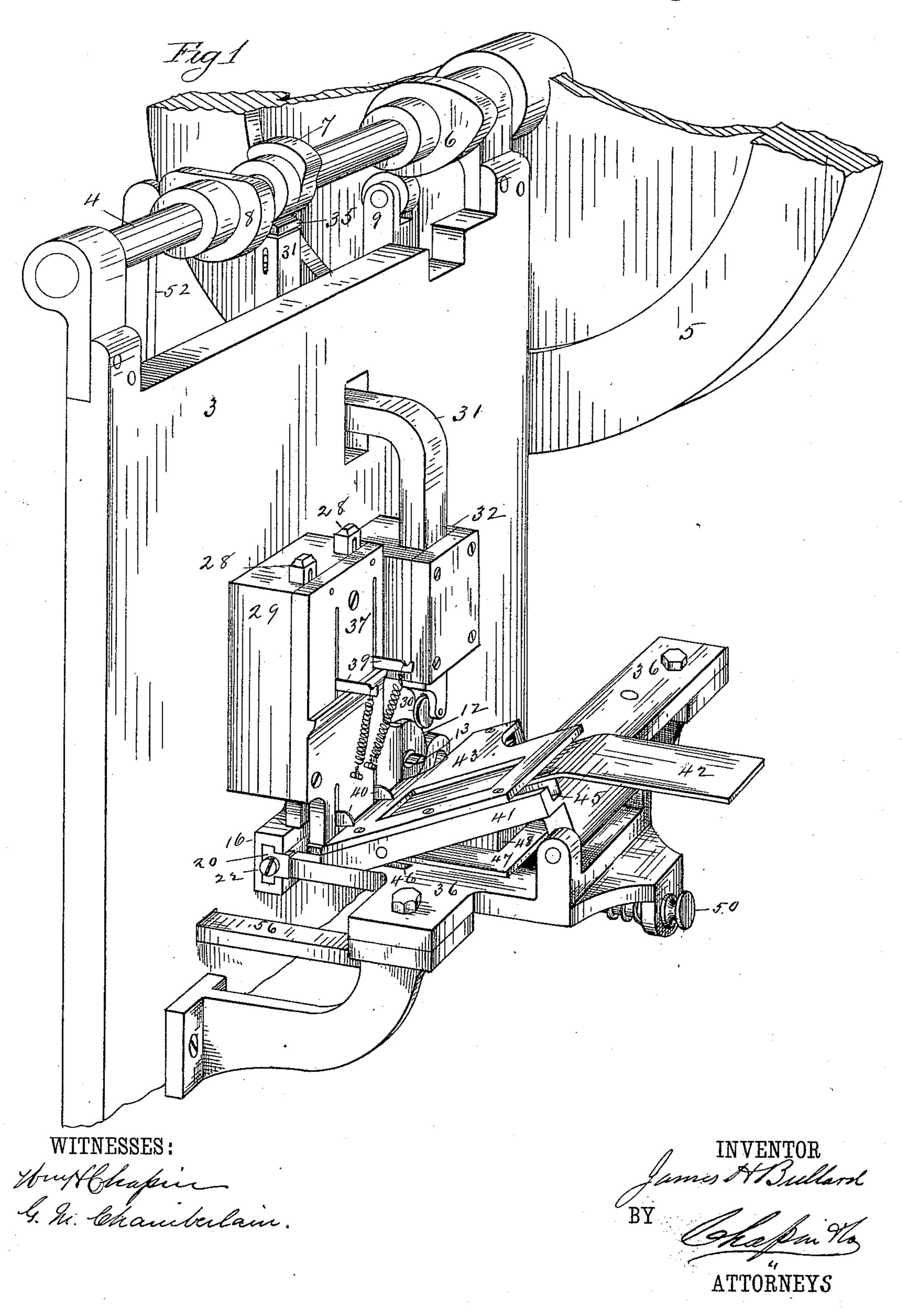
MACHINE FOR BENDING THE ENDS OF KNITTING MACHINE NEEDLES.
