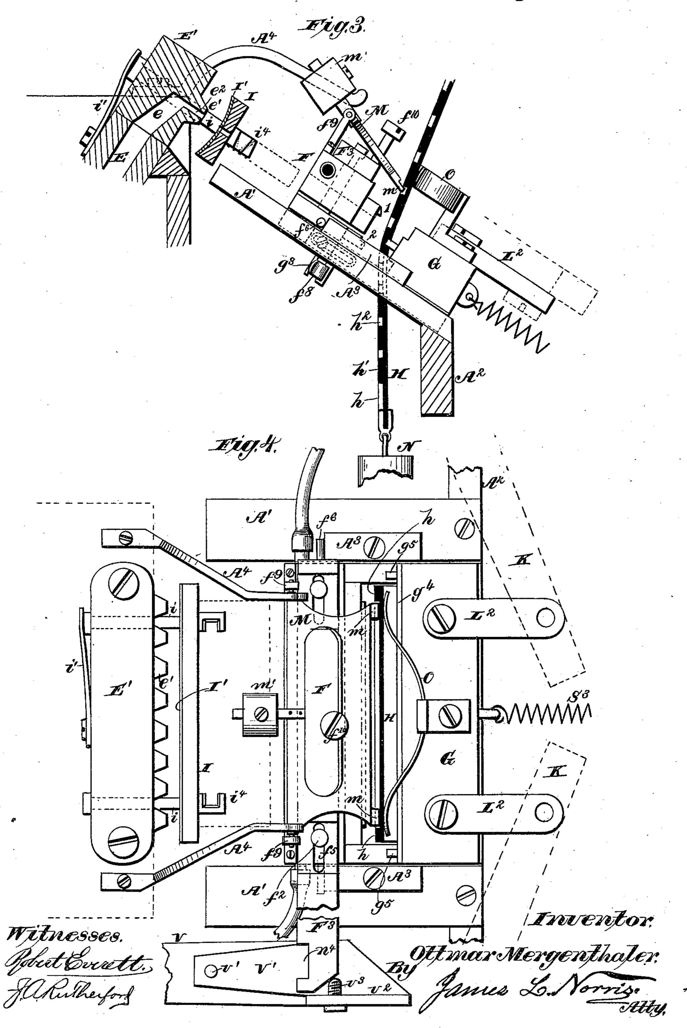
MACHINE FOR CASTING STEREOTYPES.
