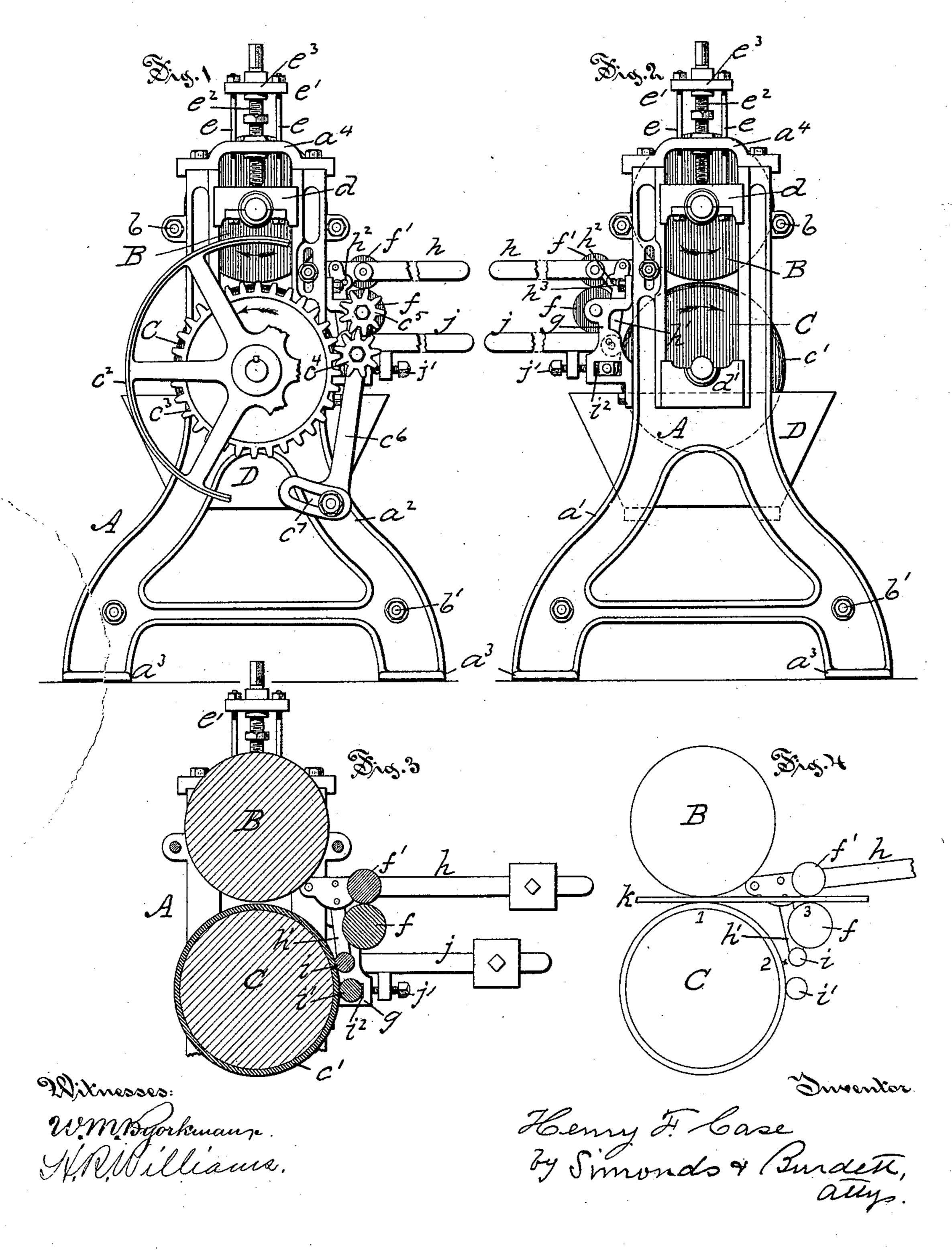
MACHINE FOR SIZING AND COLORING PAPER AND OTHER FABRICS.
