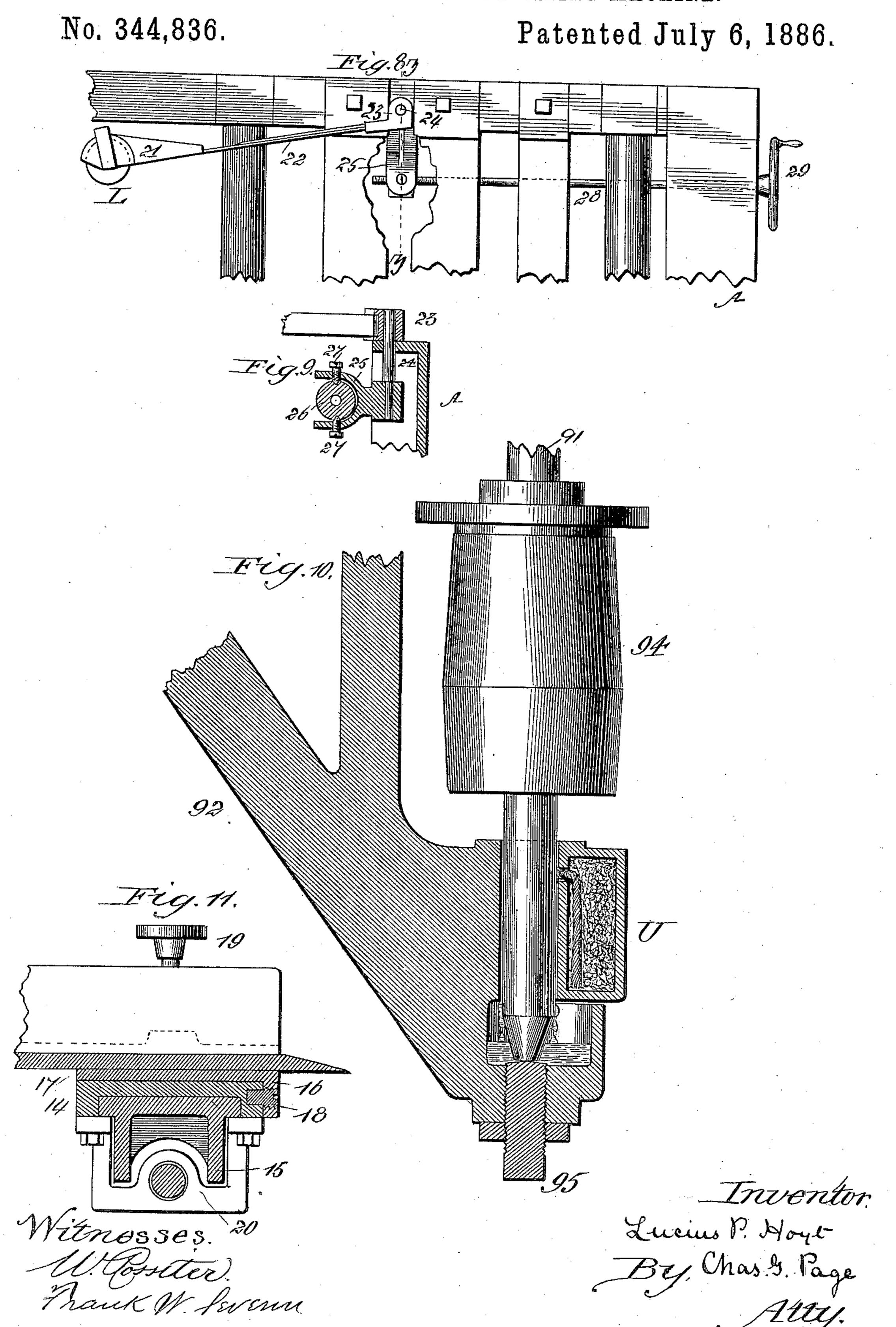
CHAIN FEED SURFACING AND SIZING MACHINE.
