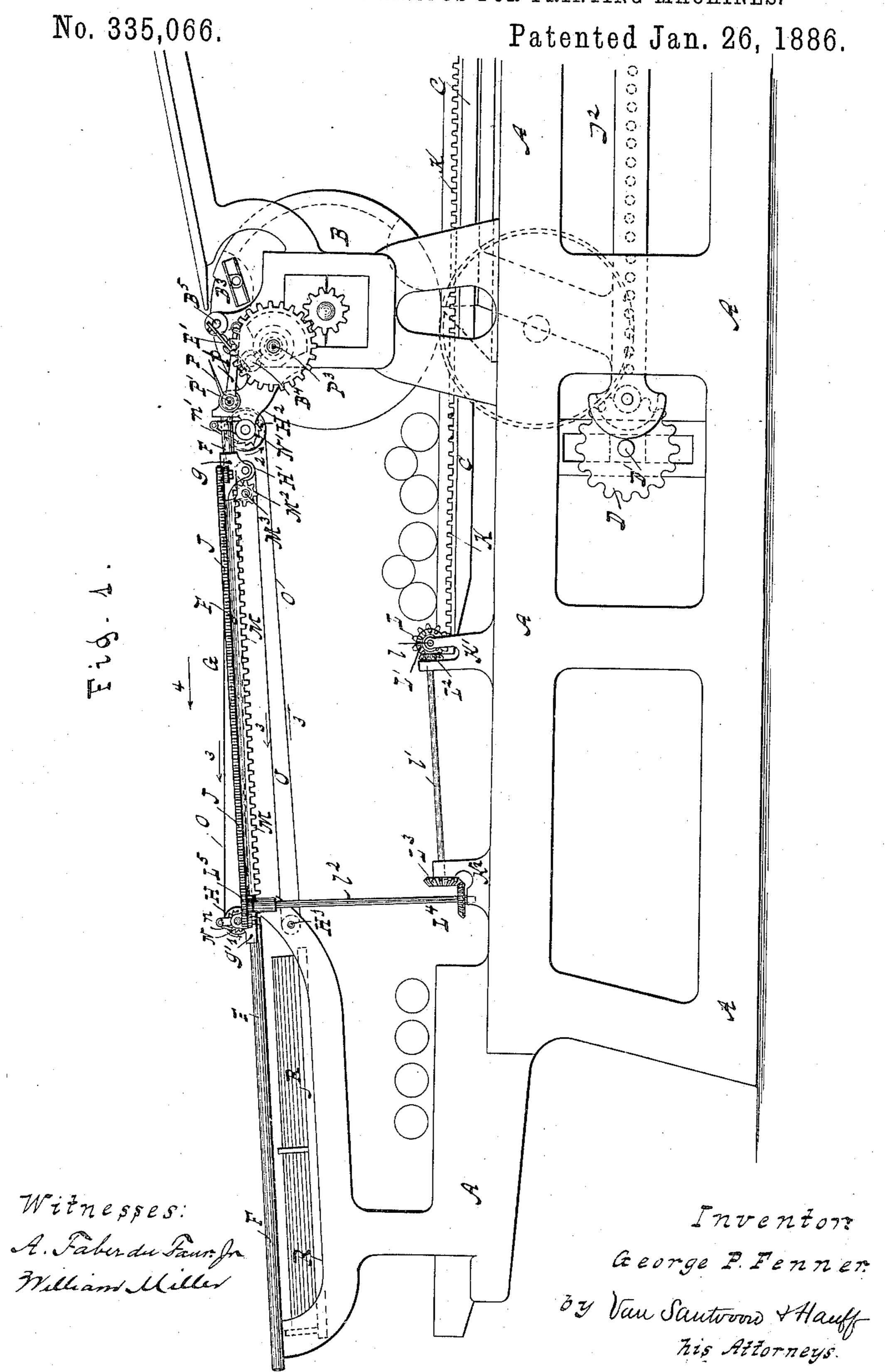
SHEET DELIVERY APPARATUS FOR PRINTING MACHINES.
