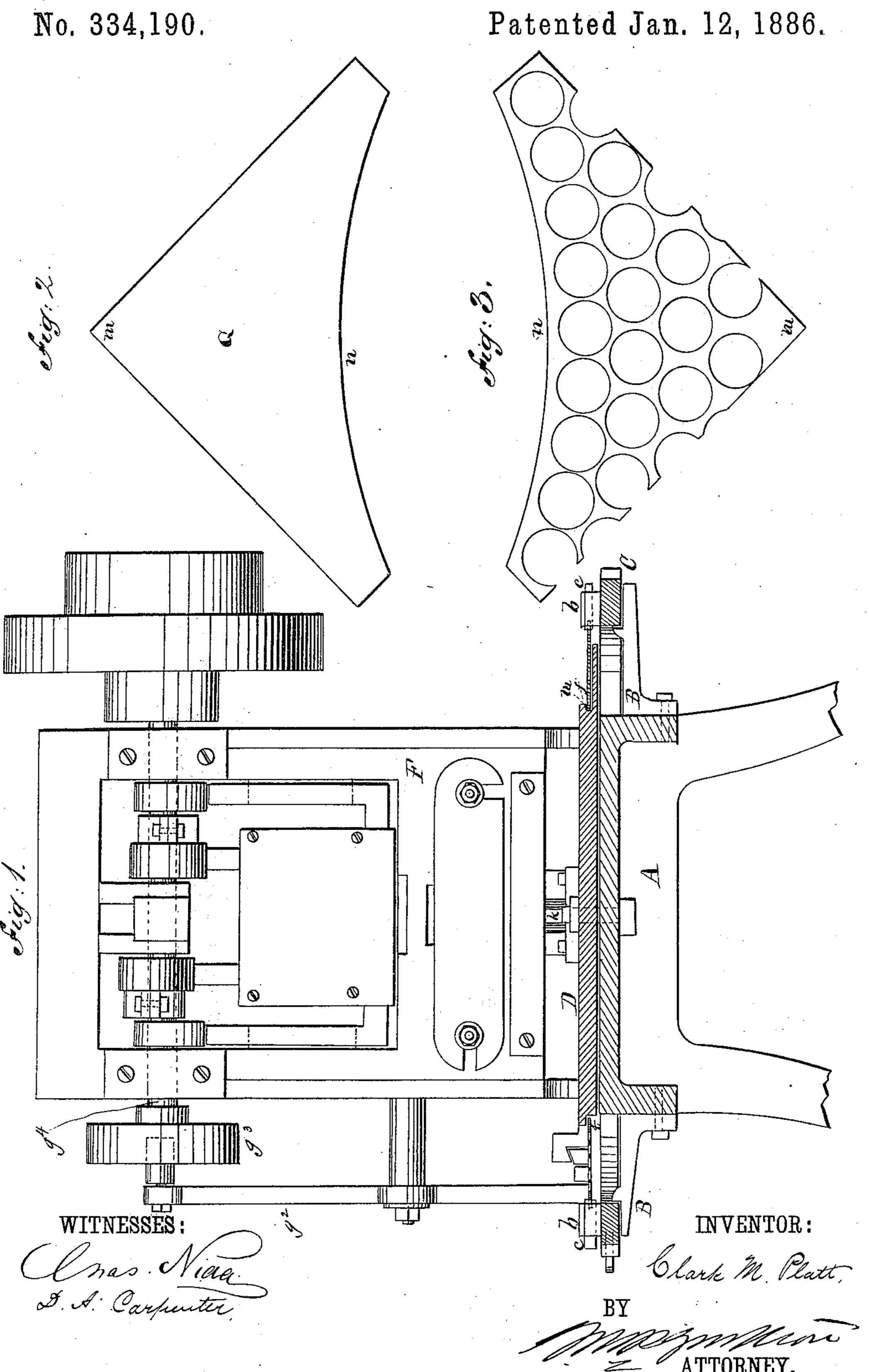
MACHINE FOR PUNCHING AND FEEDING SCRAPS OF SHEET METAL.
