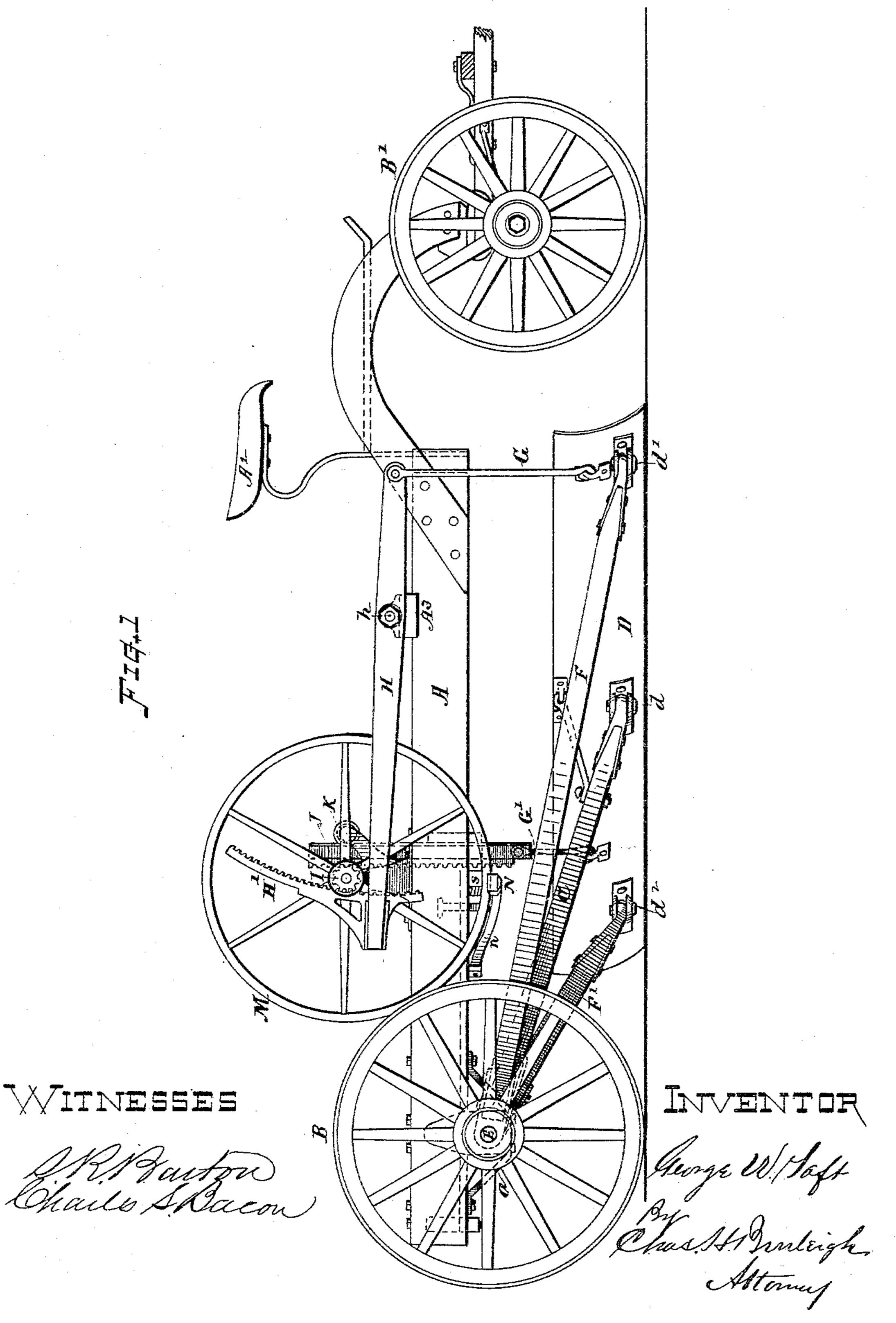
MACHINE FOR MAKING, REPAIRING, AND CLEANING ROADS.
