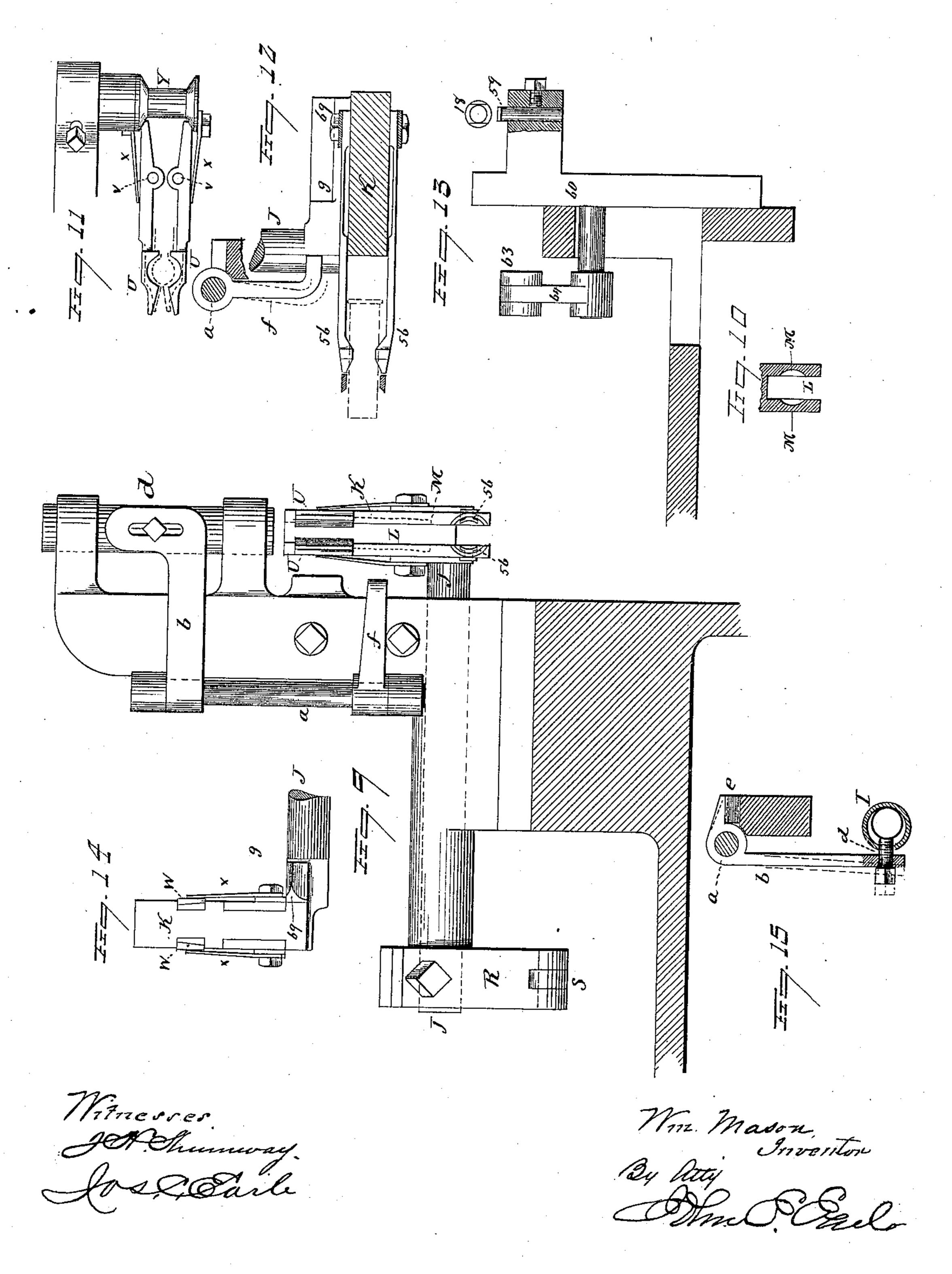
MACHINE FOR TRIMMING CARTRIDGE SHELLS.
