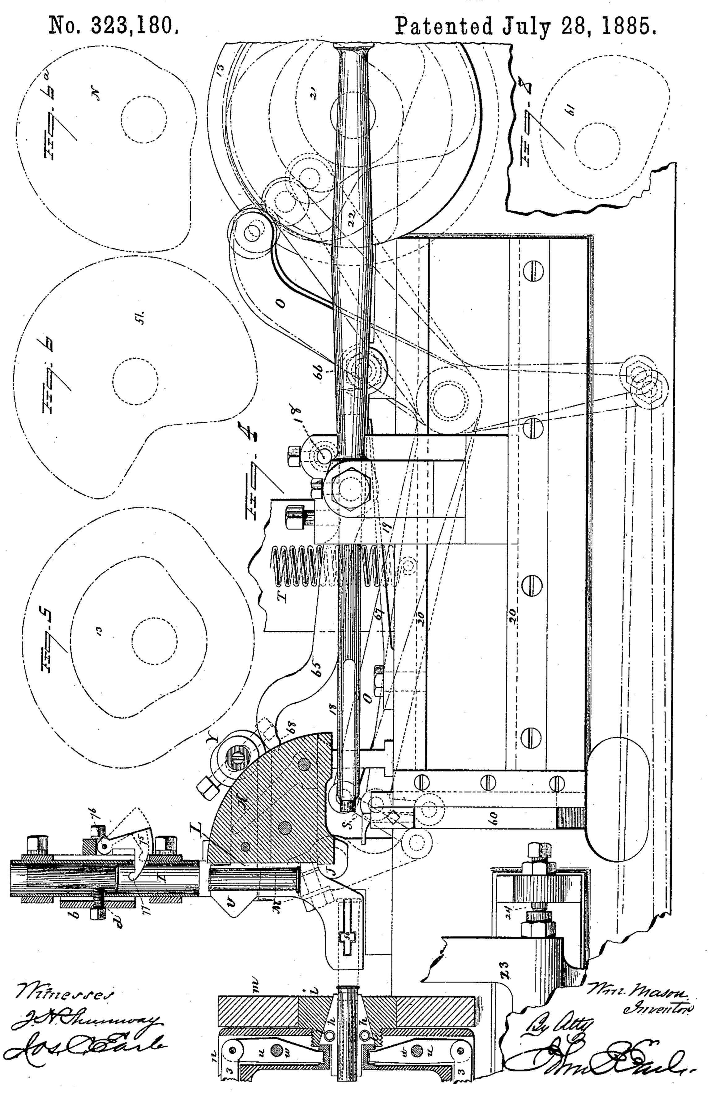
MACHINE FOR TRIMMING CARTRIDGE SHELLS.
