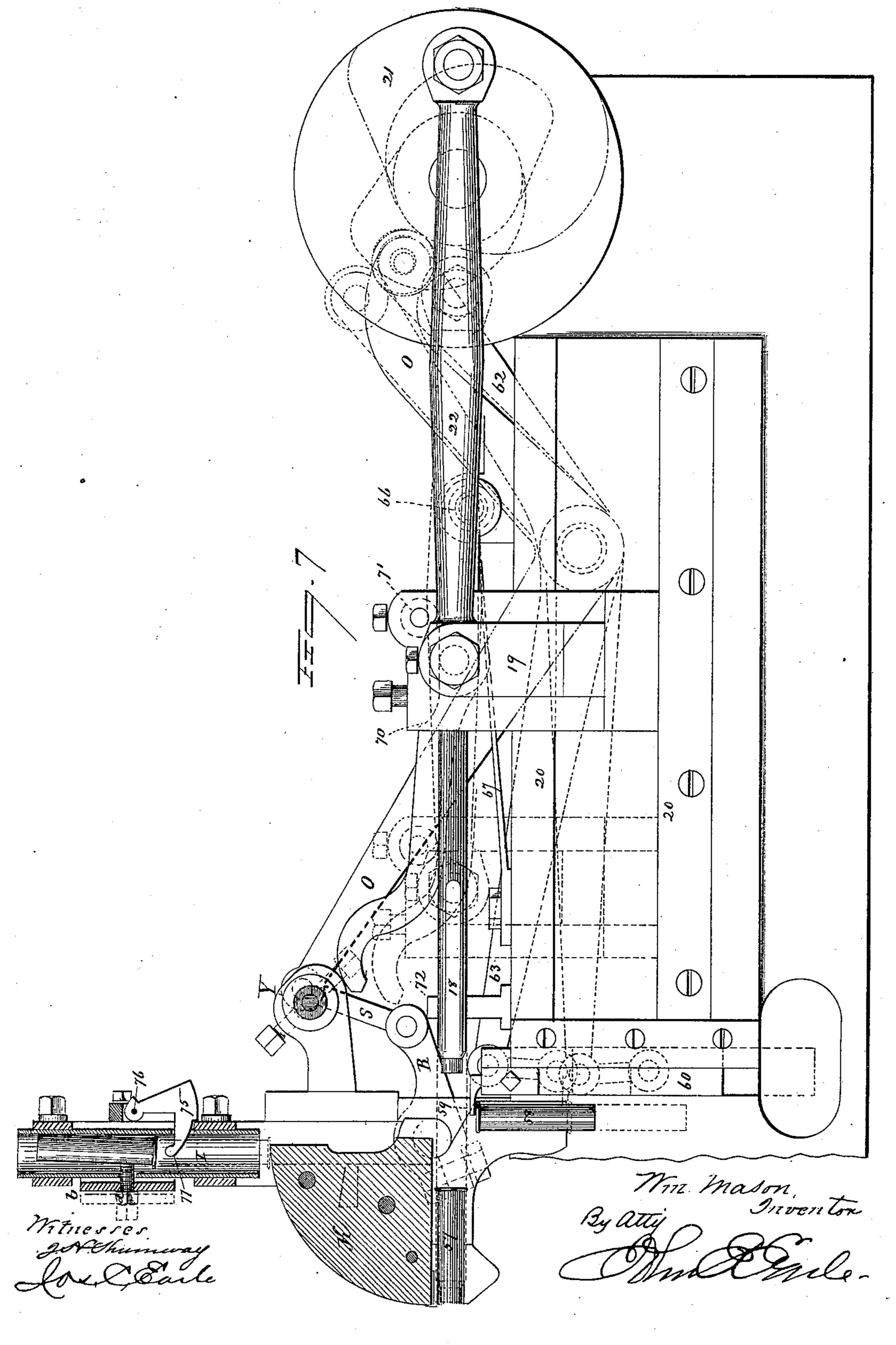
MACHINE FOR TRIMMING CARTRIDGE SHELLS.
