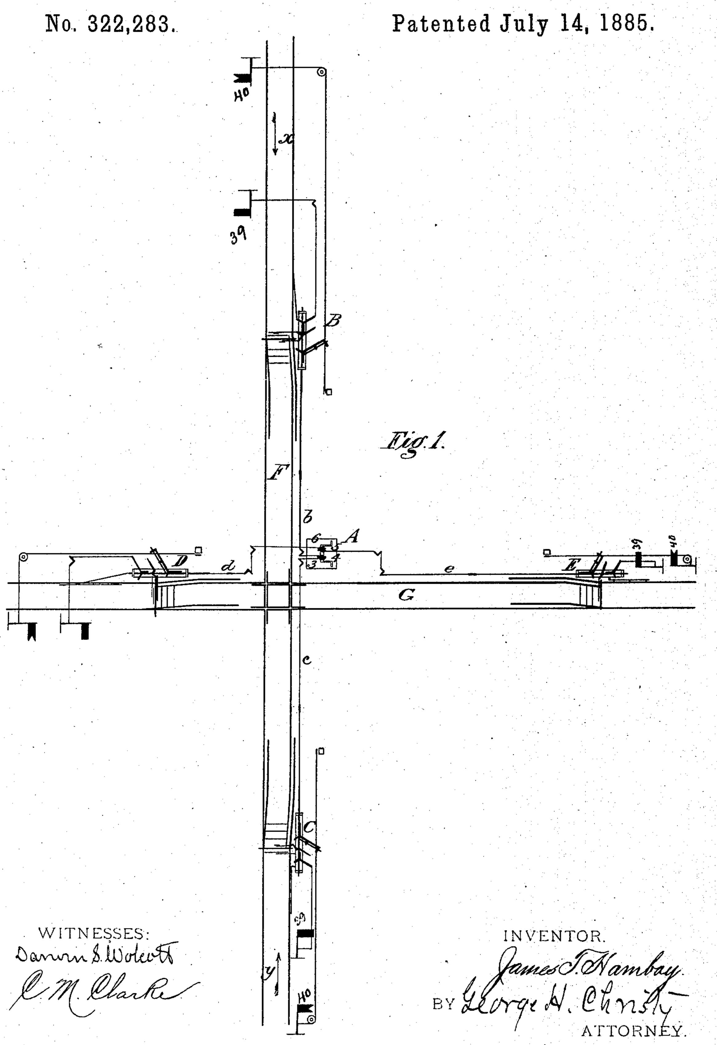
INTERLOCKING SWITCH AND SIGNAL APPARATUS.
