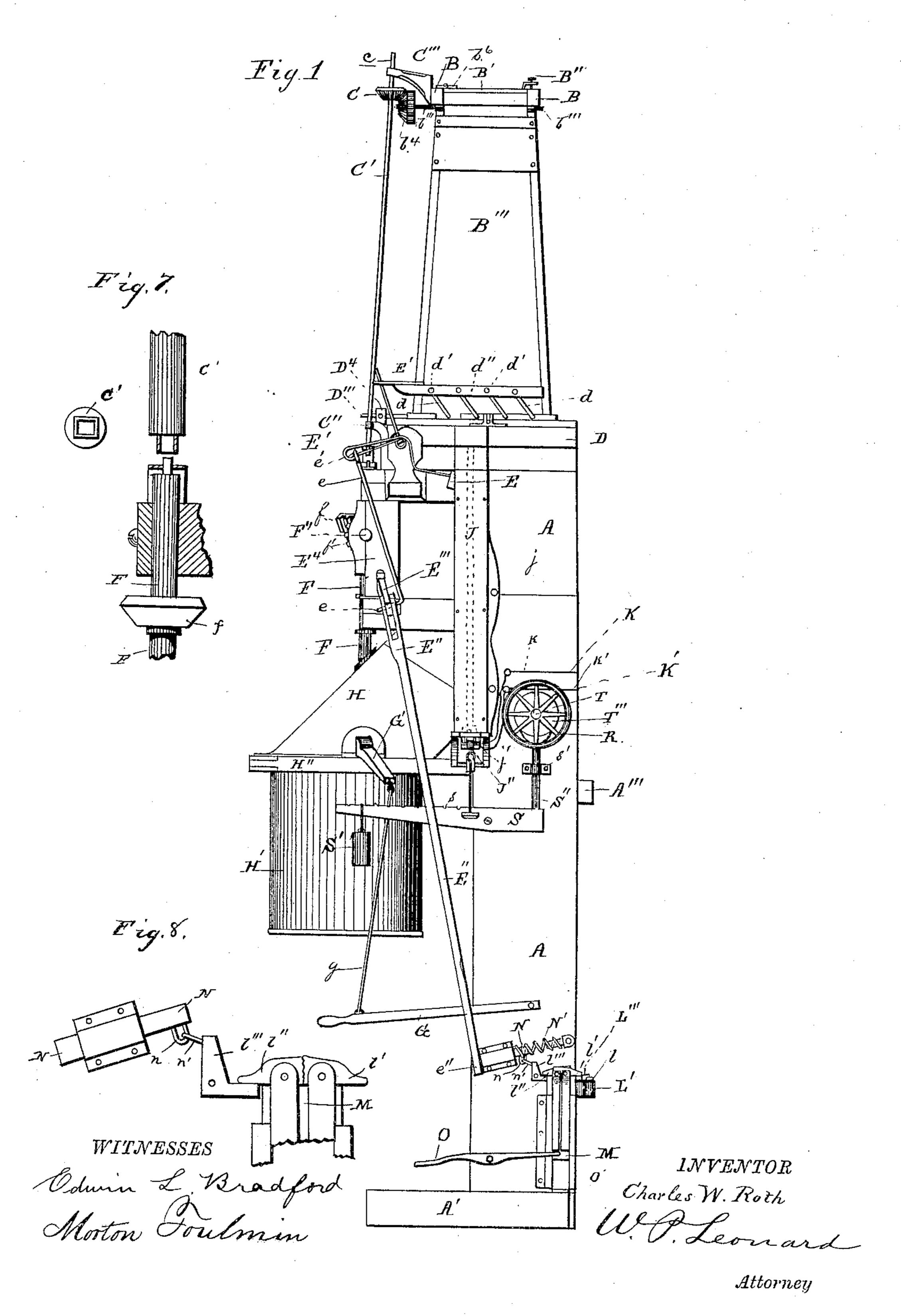
COMBINED ELECTRICAL WEIGHING SCALE AND FLOUR AND BRAN PACKER.
