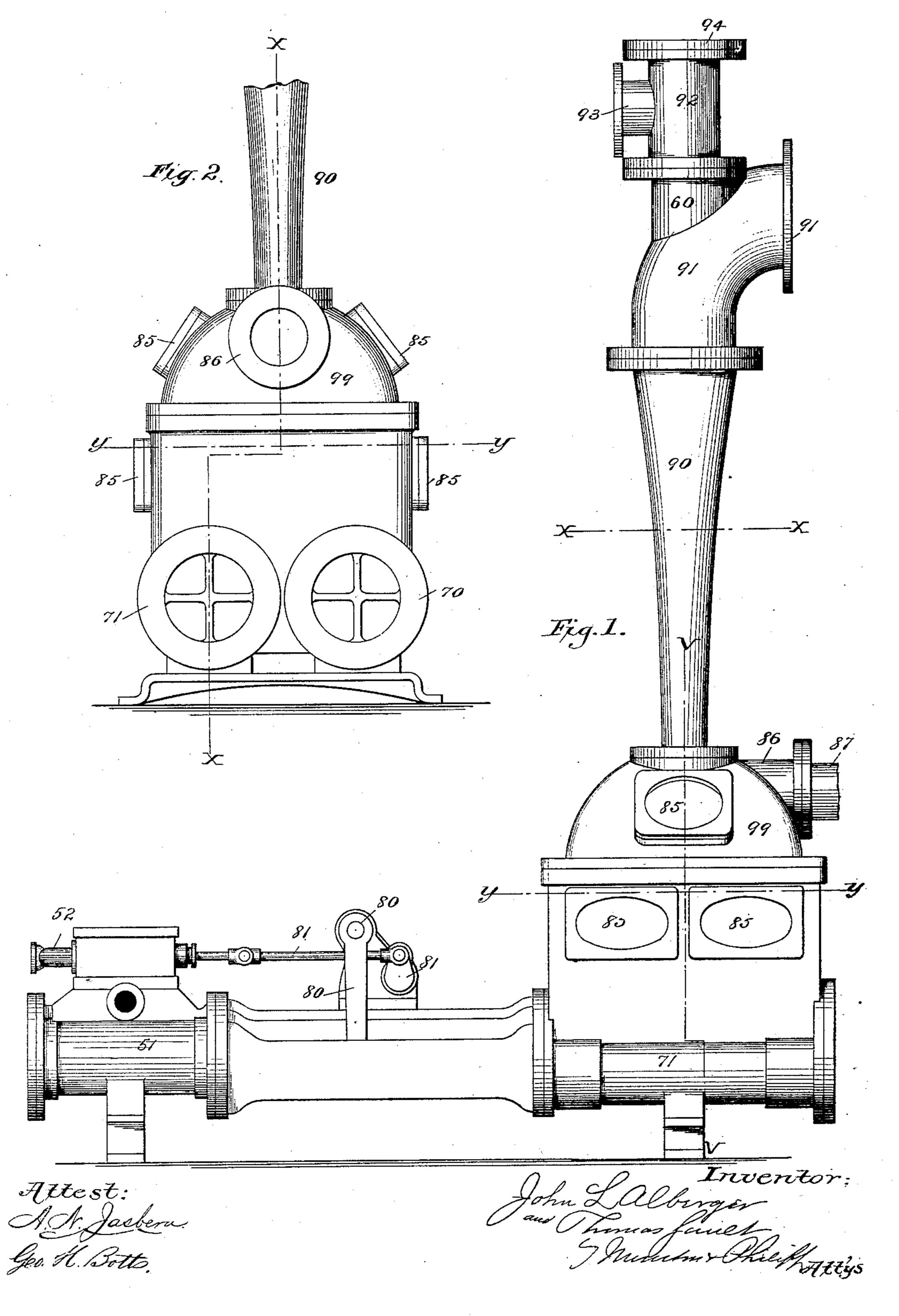
CONDENSING APPARATUS FOR STEAM ENGINES.
