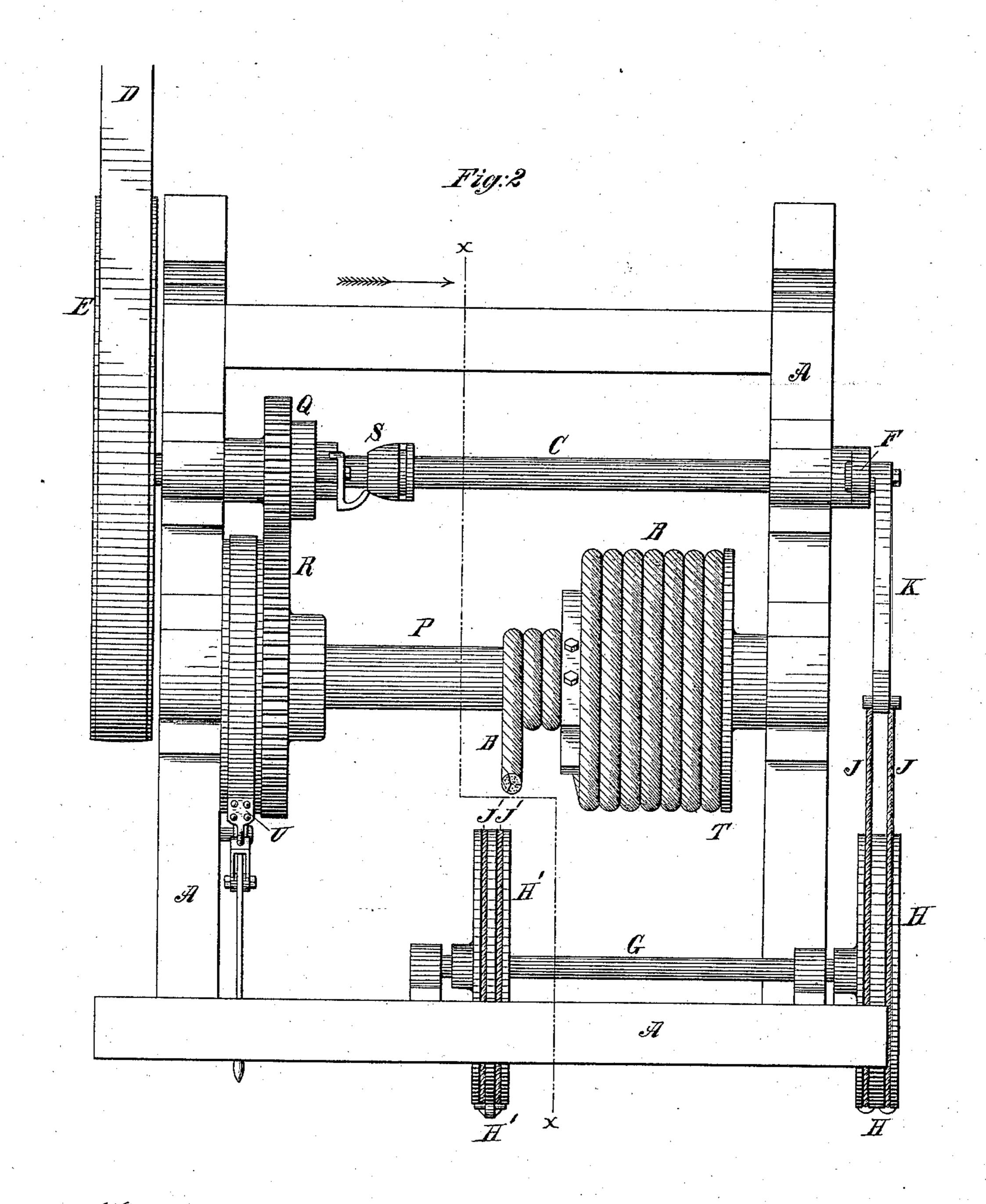
ROCK DRILLING MACHINE FOR ARTESIAN WELLS.
