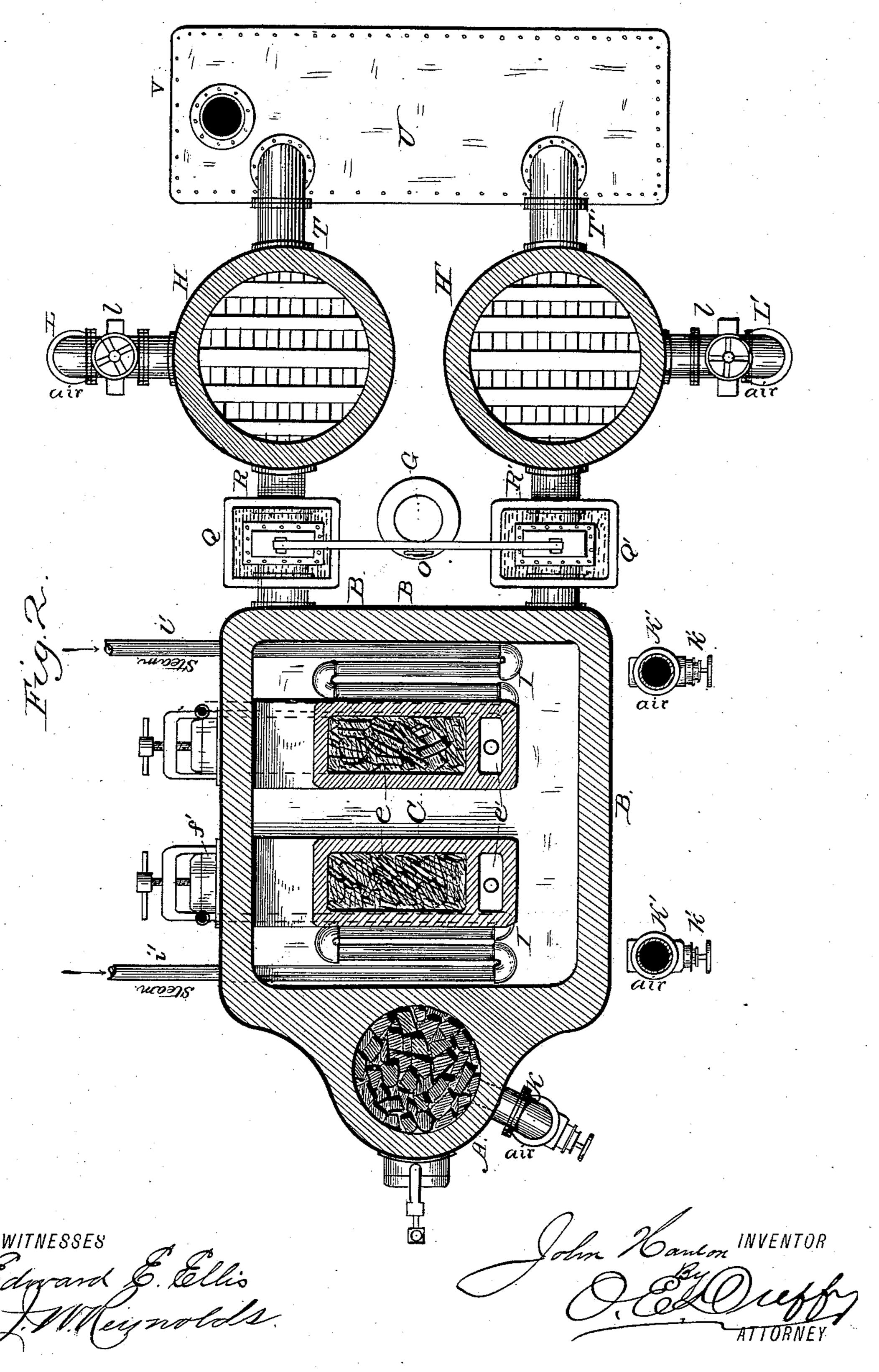
PROCESS OF AND APPARATUS FOR MANUFACTURING GAS.
