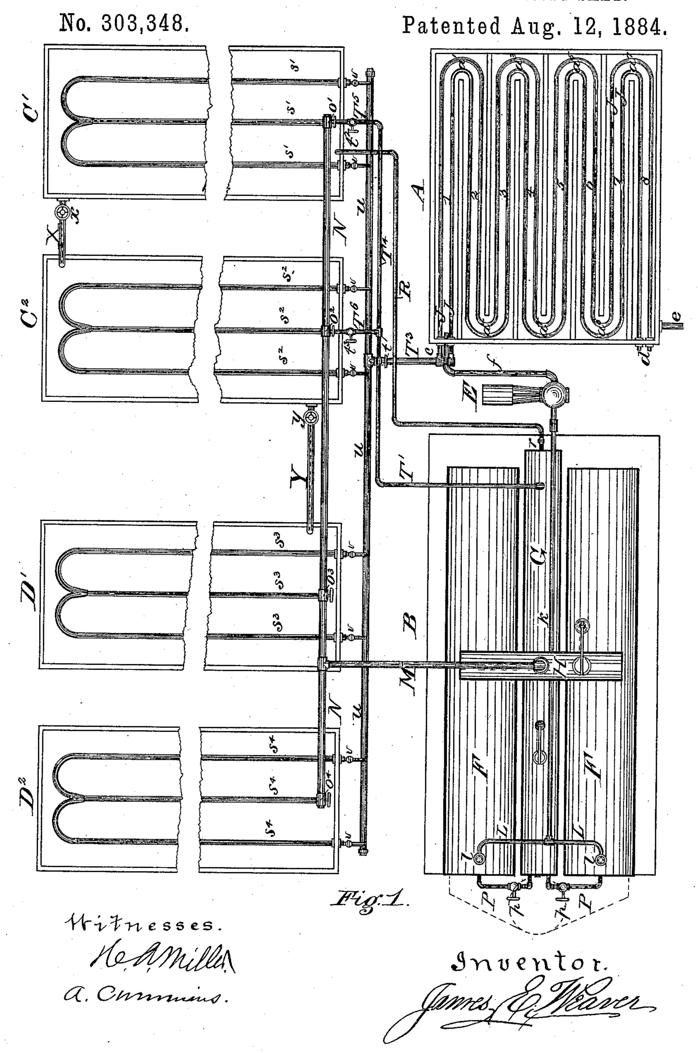
PROCESS OF AND APPARATUS FOR MANUFACTURING SALT.
