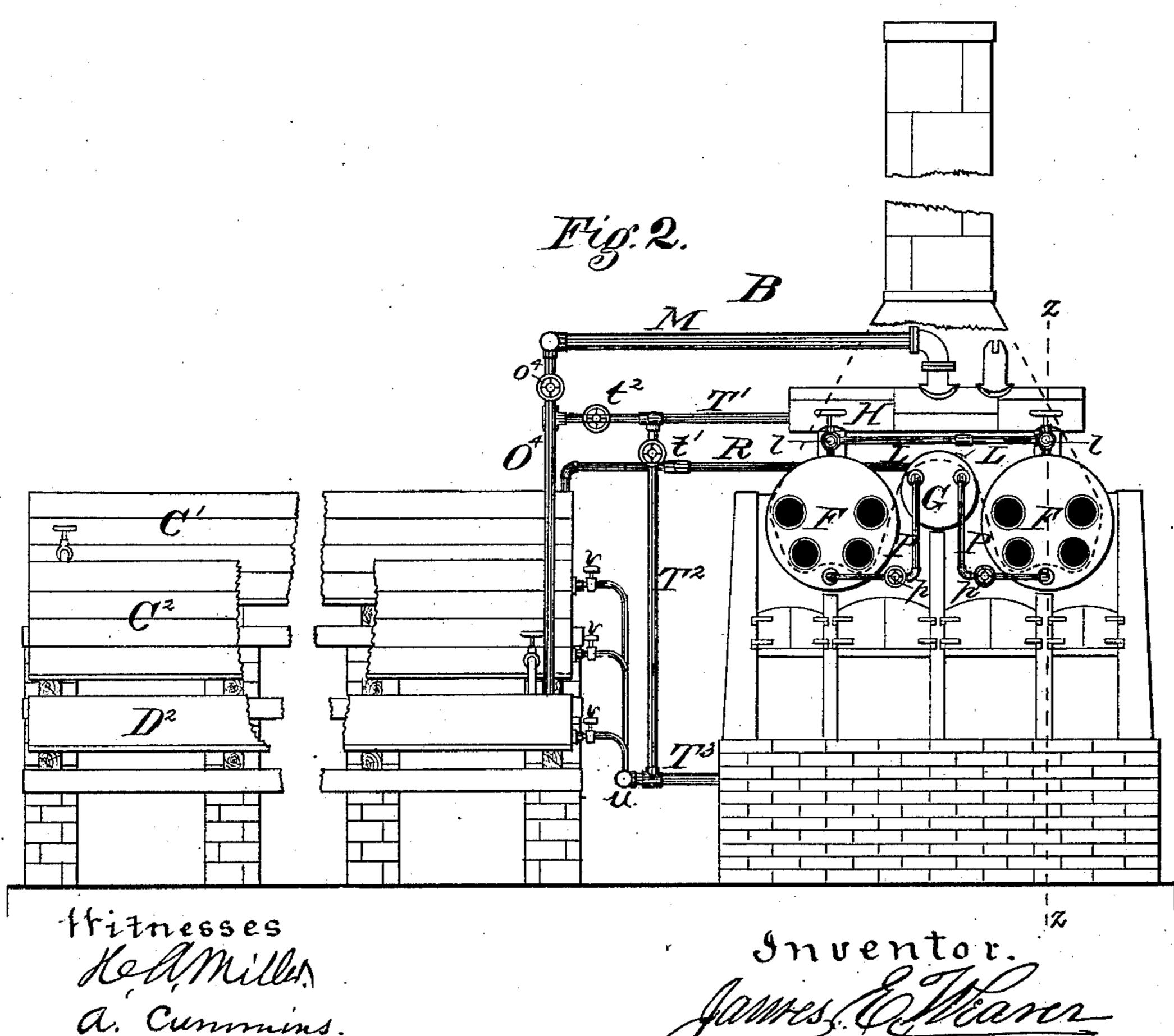
PROCESS OF AND APPARATUS FOR MANUFACTURING SALT.
