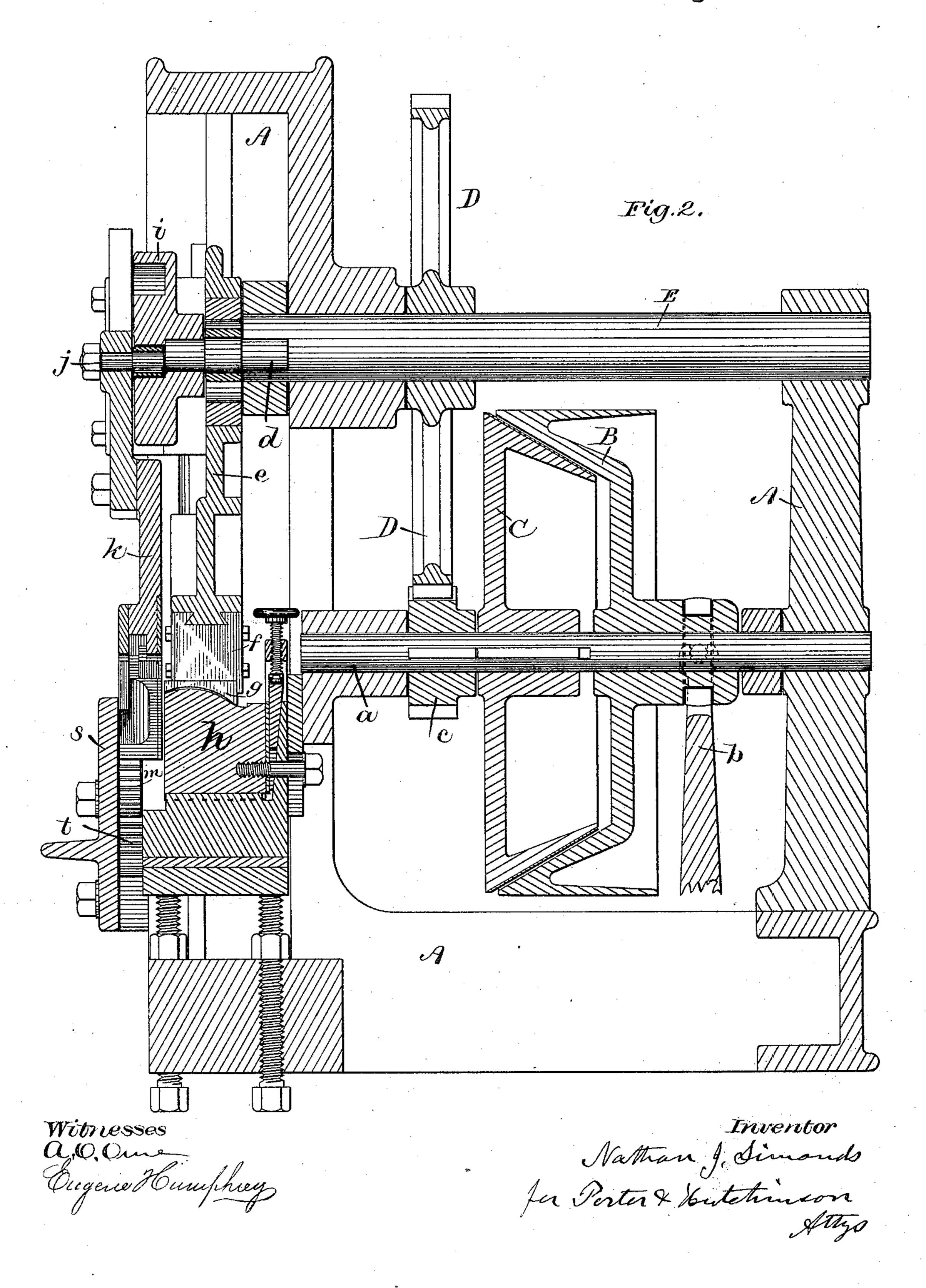
MACHINE FOR MOLDING BOOT OR SHOE STIFFENERS.
