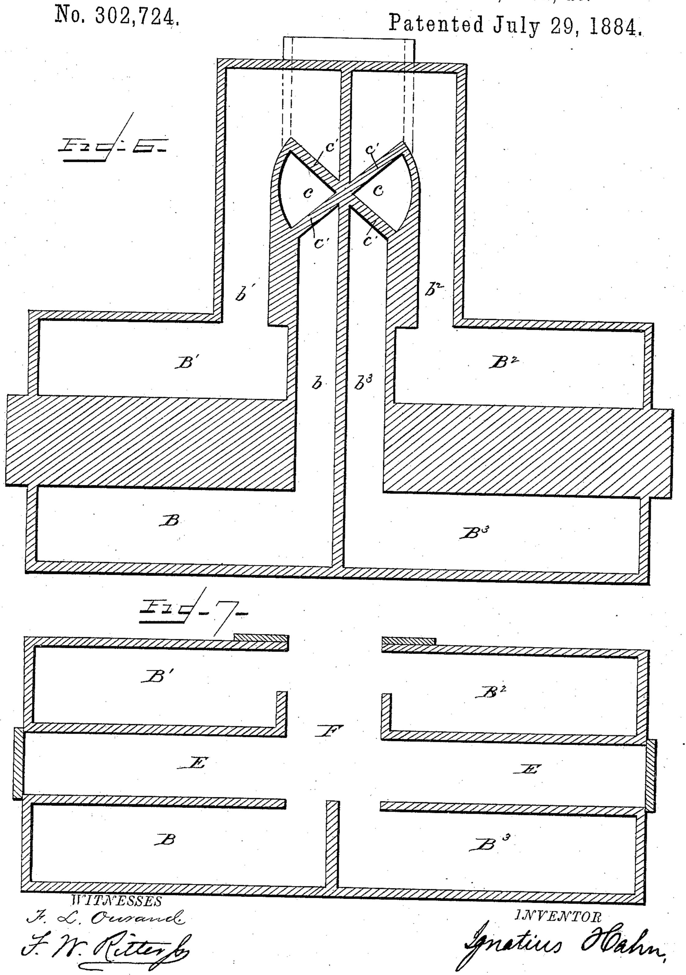
FURNACE FOR THE MANUFACTURE OF GLASS, IRON, &c.
