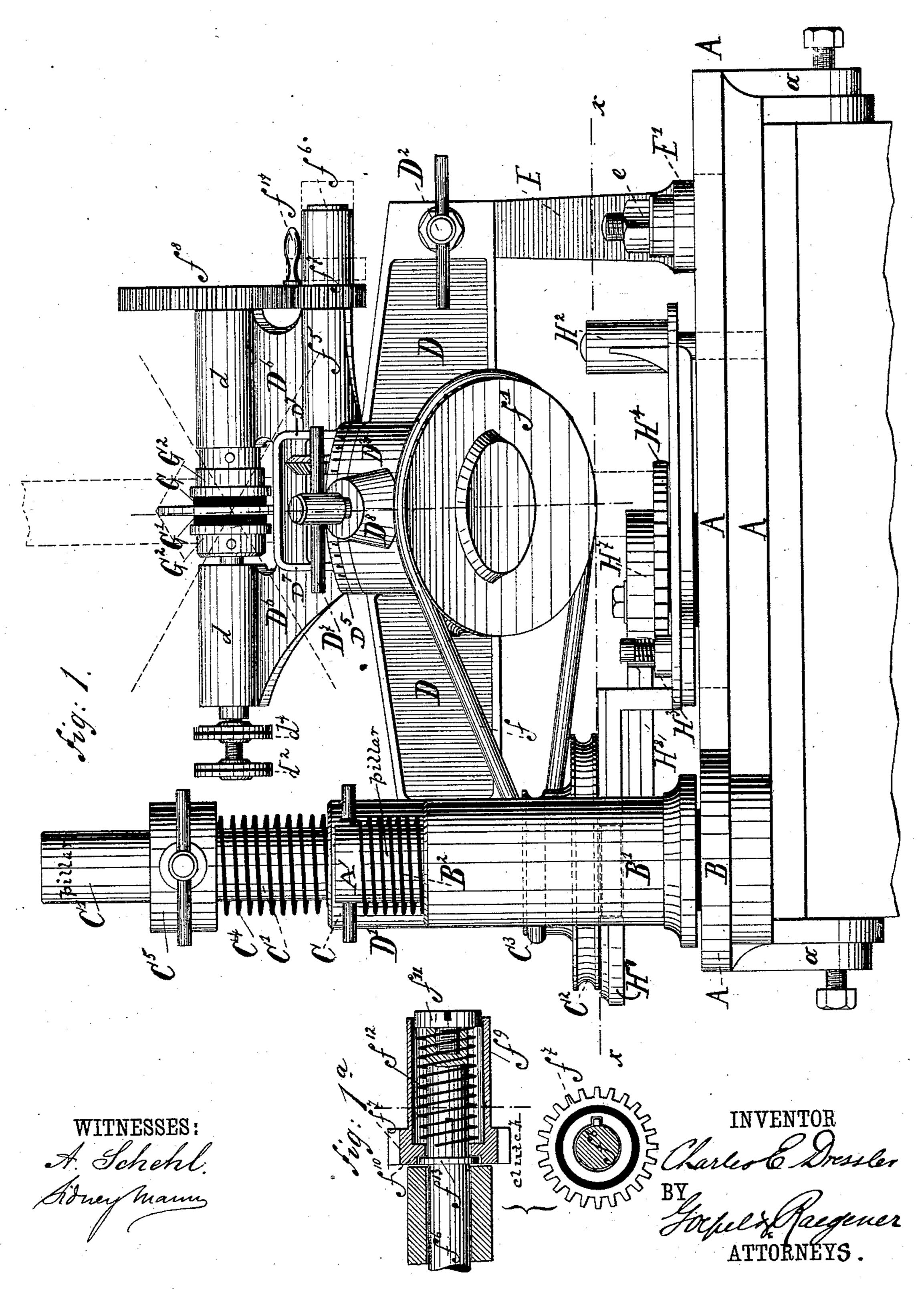
MACHINE FOR GRINDING THE RIMS OF LENSES.
