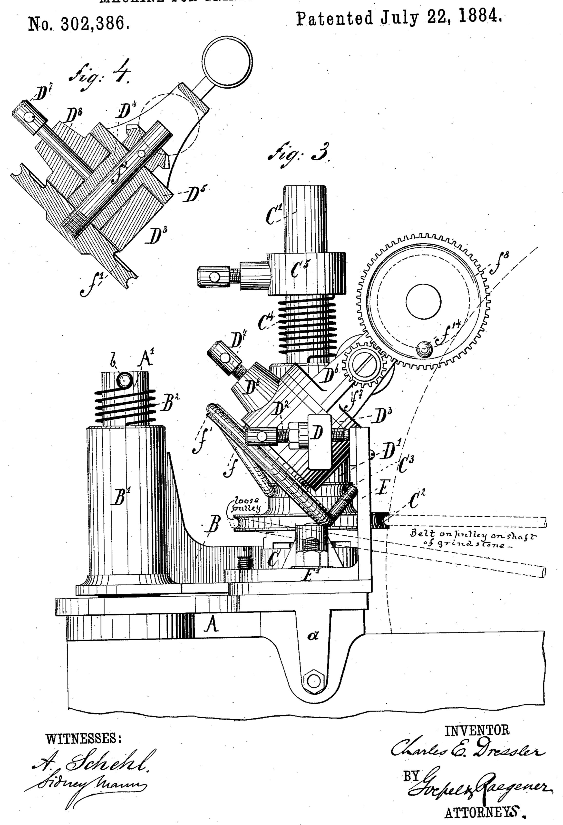
MACHINE FOR GRINDING THE RIMS OF LENSES.
