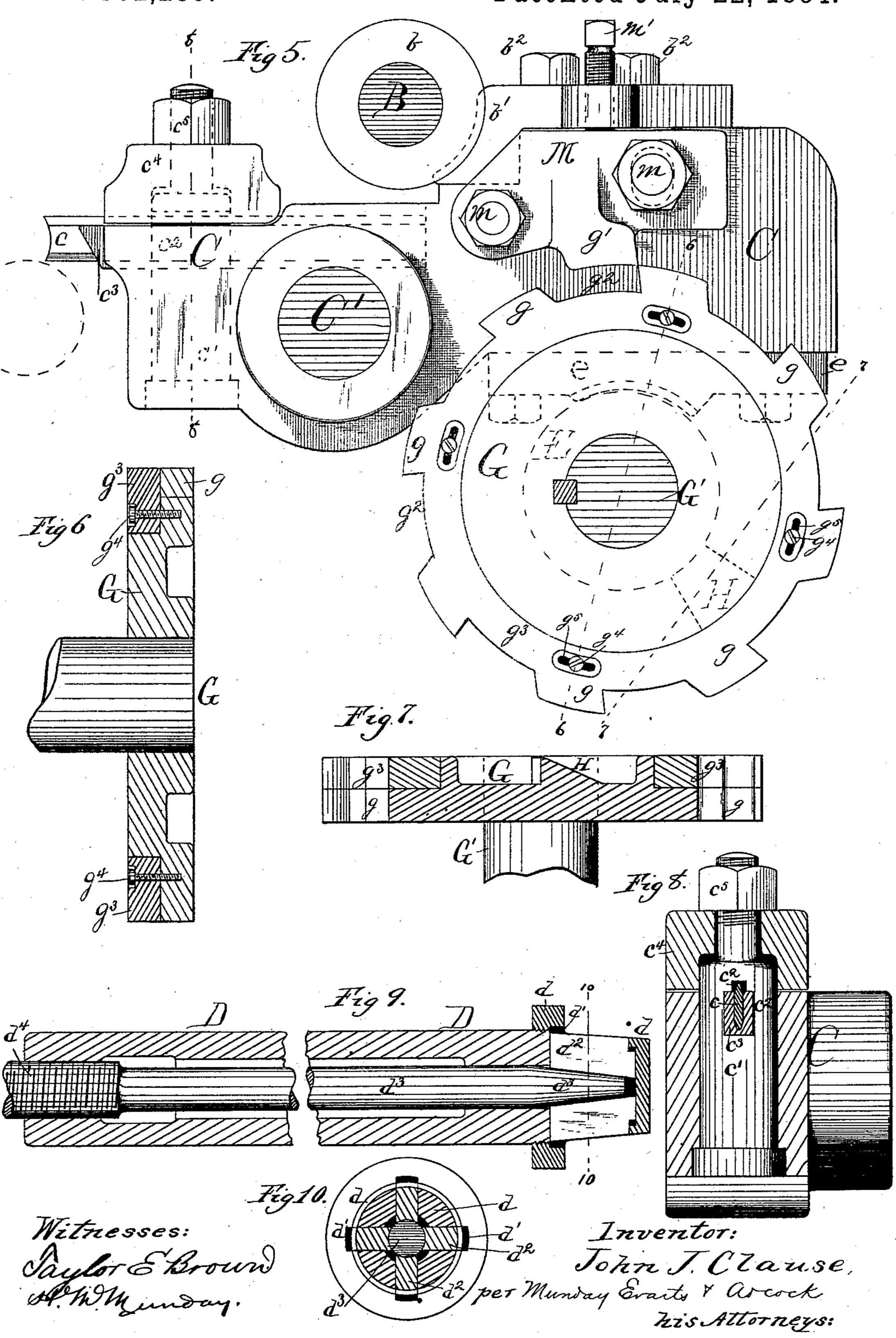
MACHINE FOR CUTTING SCREW THREADS UPON CONICAL ARTICLES.
