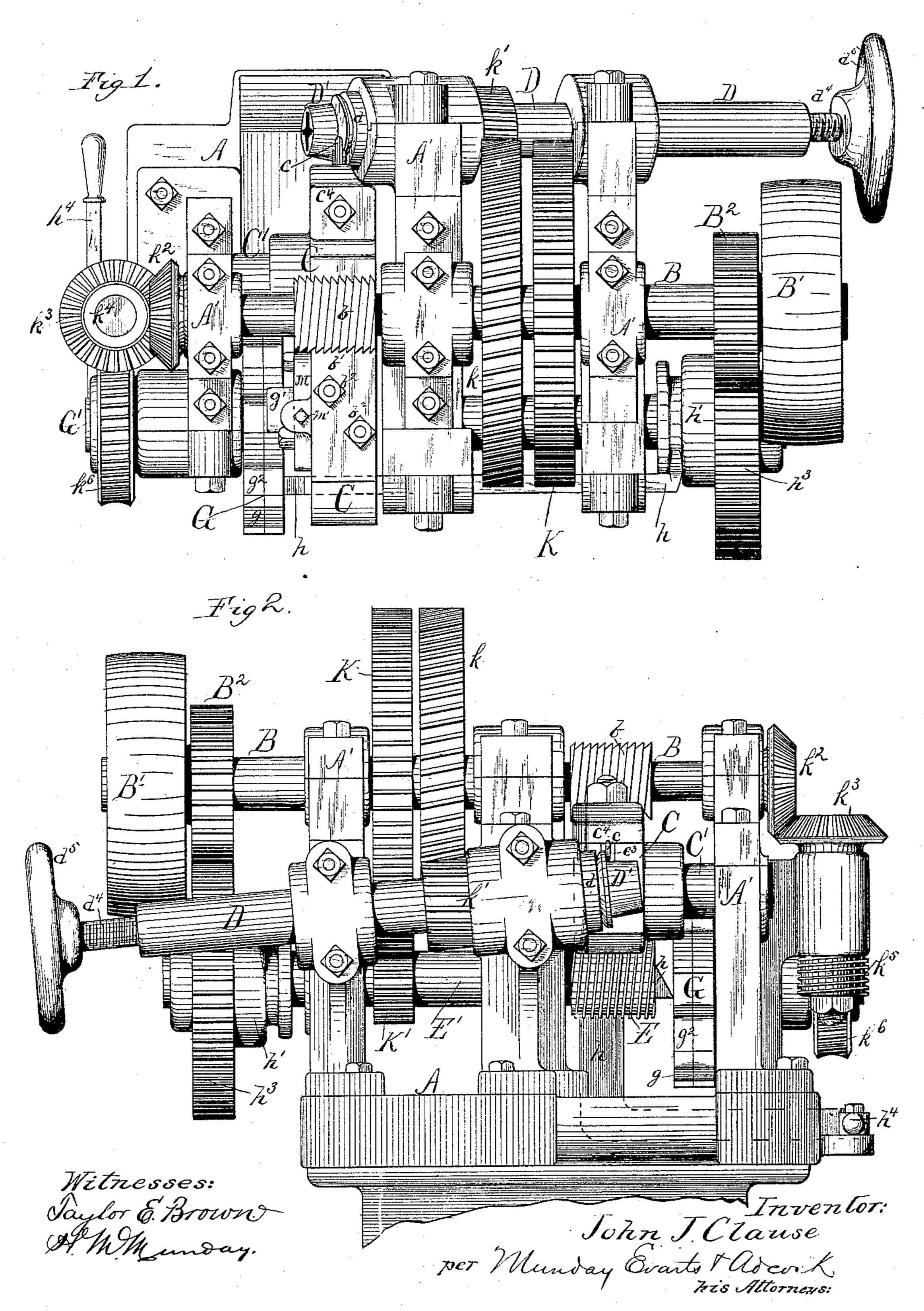
MACHINE FOR CUTTING SCREW THREADS UPON CONICAL ARTICLES.
