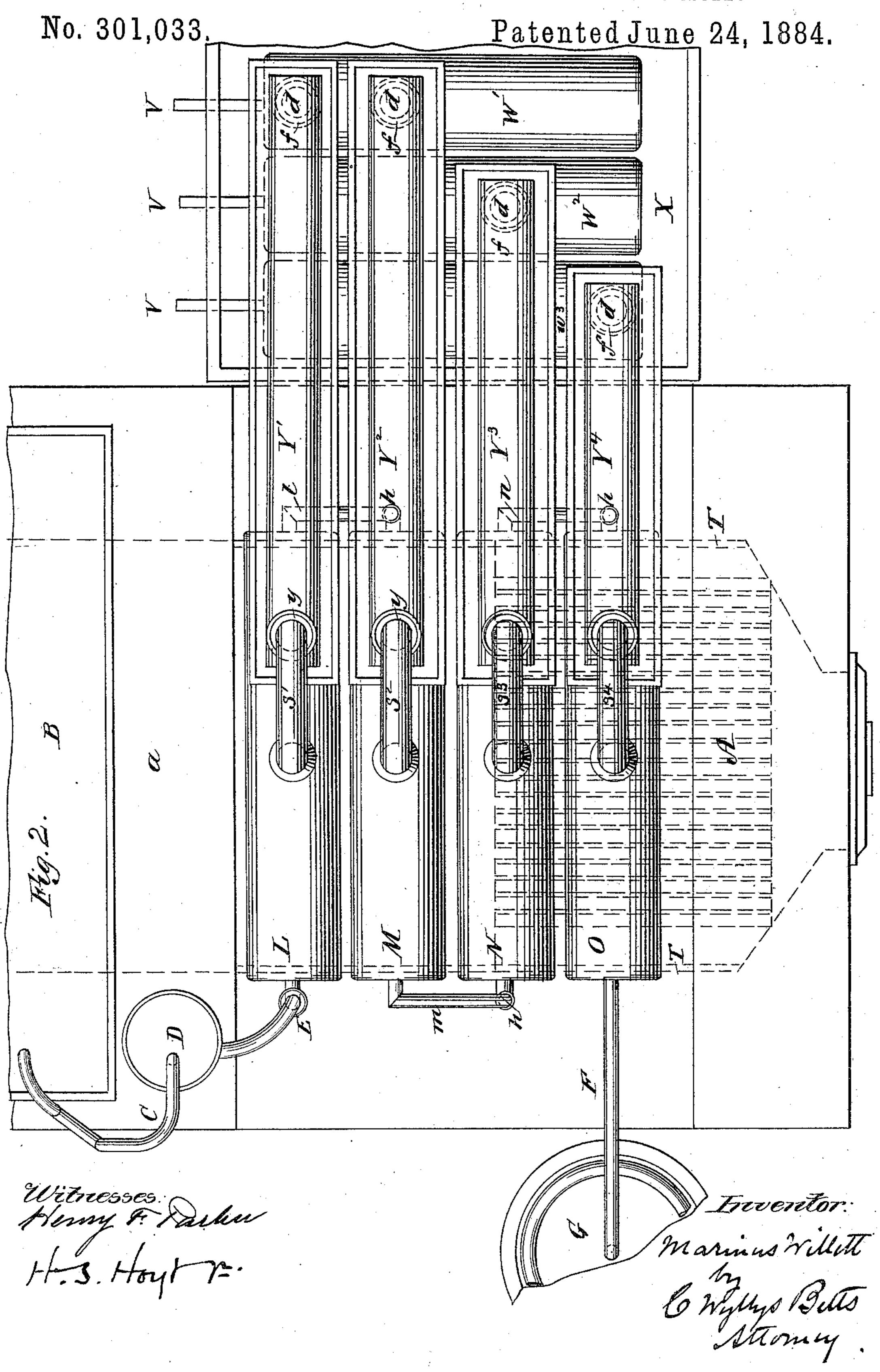
APPARATUS FOR CONCENTRATING SULPHURIC ACID.
