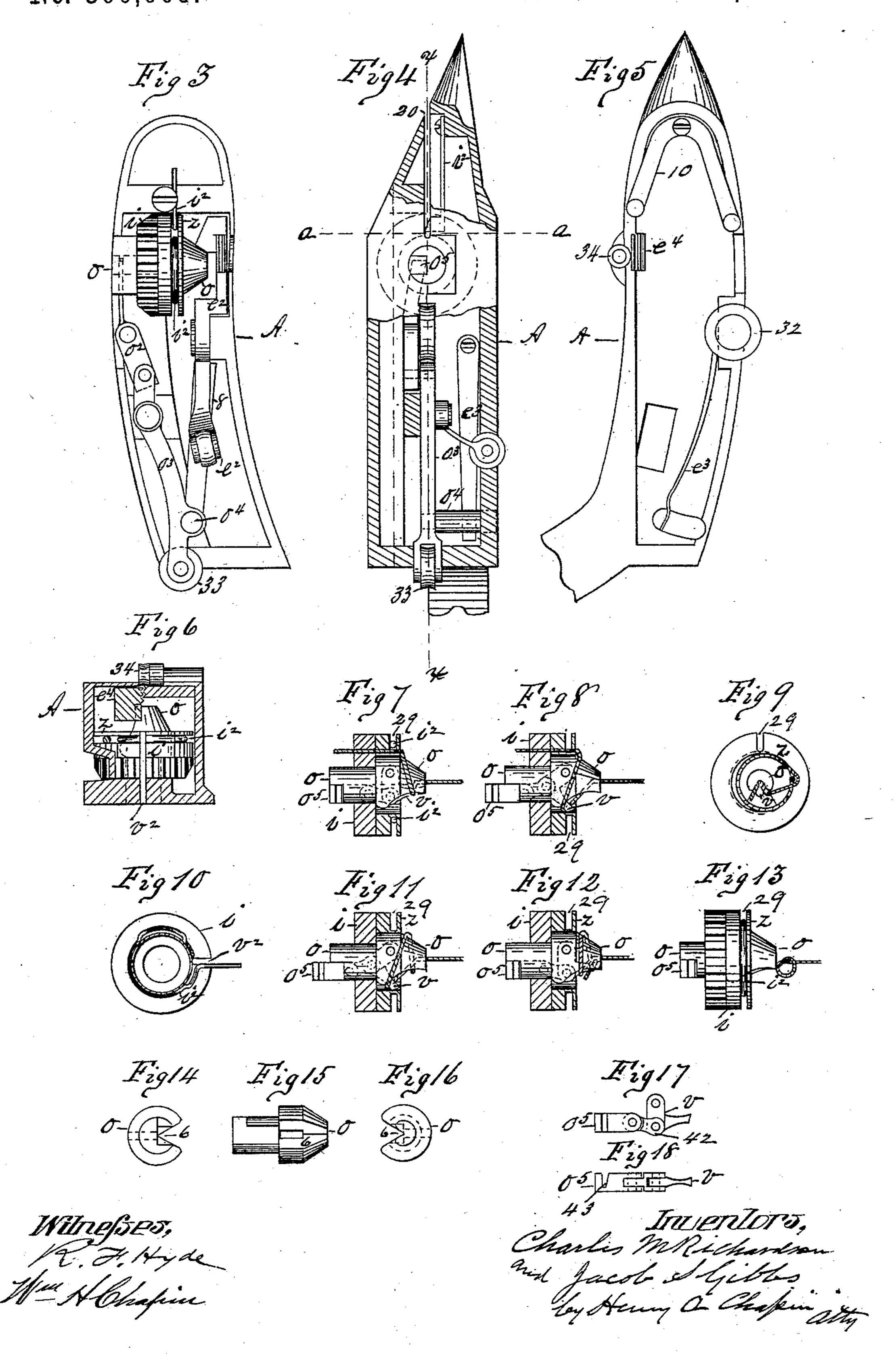
C. M. RICHARDSON & J. S. GIBBS. KNOT TYING MECHANISM FOR GRAIN BINDERS. Patented June 10, 1884.
