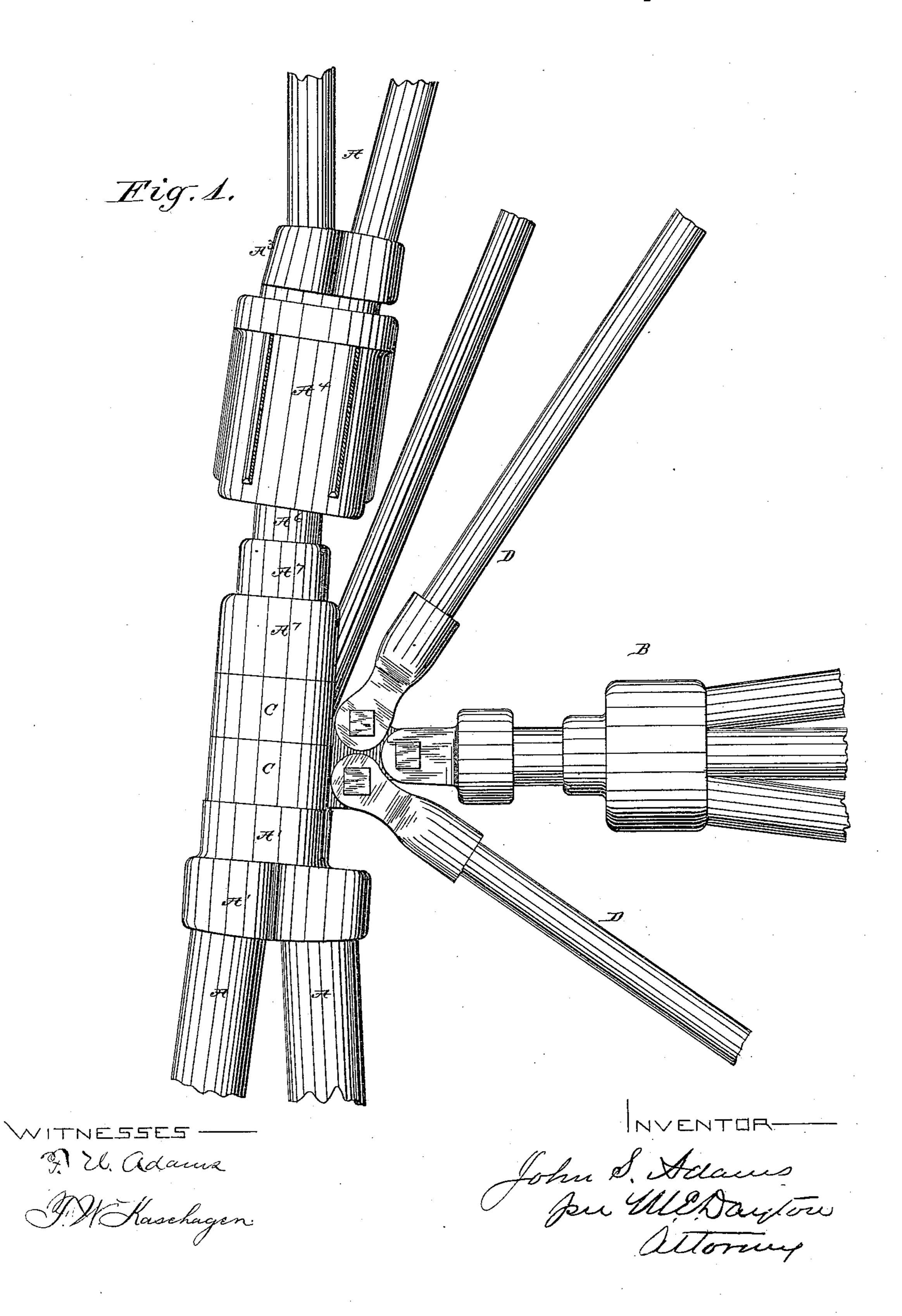
SKELETON IRON TOWER AND MODE OF ERECTING THE SAME.
