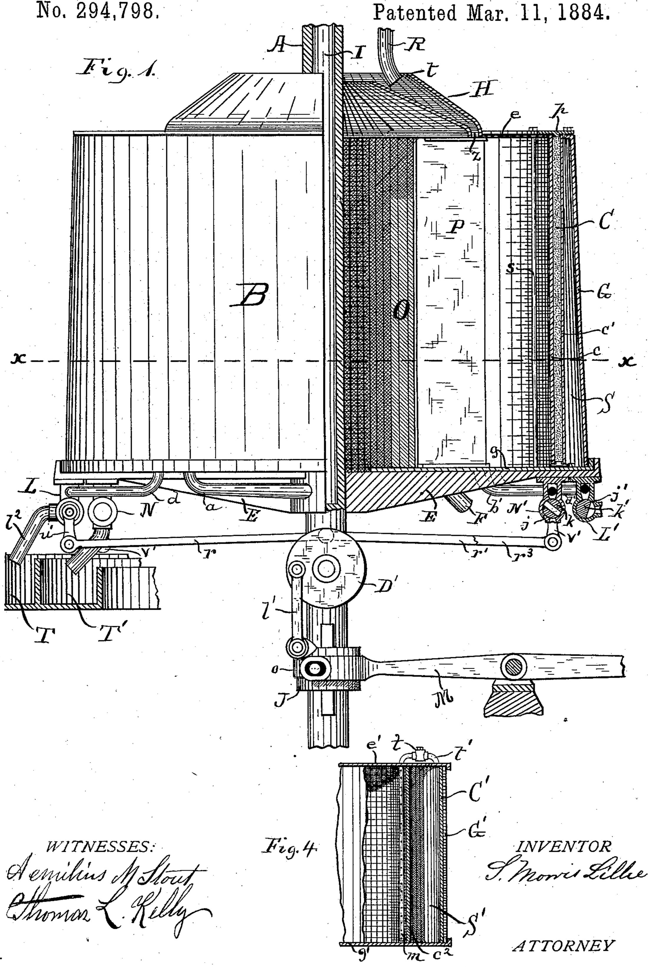
PROCESS OF AND APPARATUS FOR SEPARATING RAW SUGAR LIQUOR FROM THE SCUM AND MECHANICAL IMPURITIES CONTAINED THEREIN.
