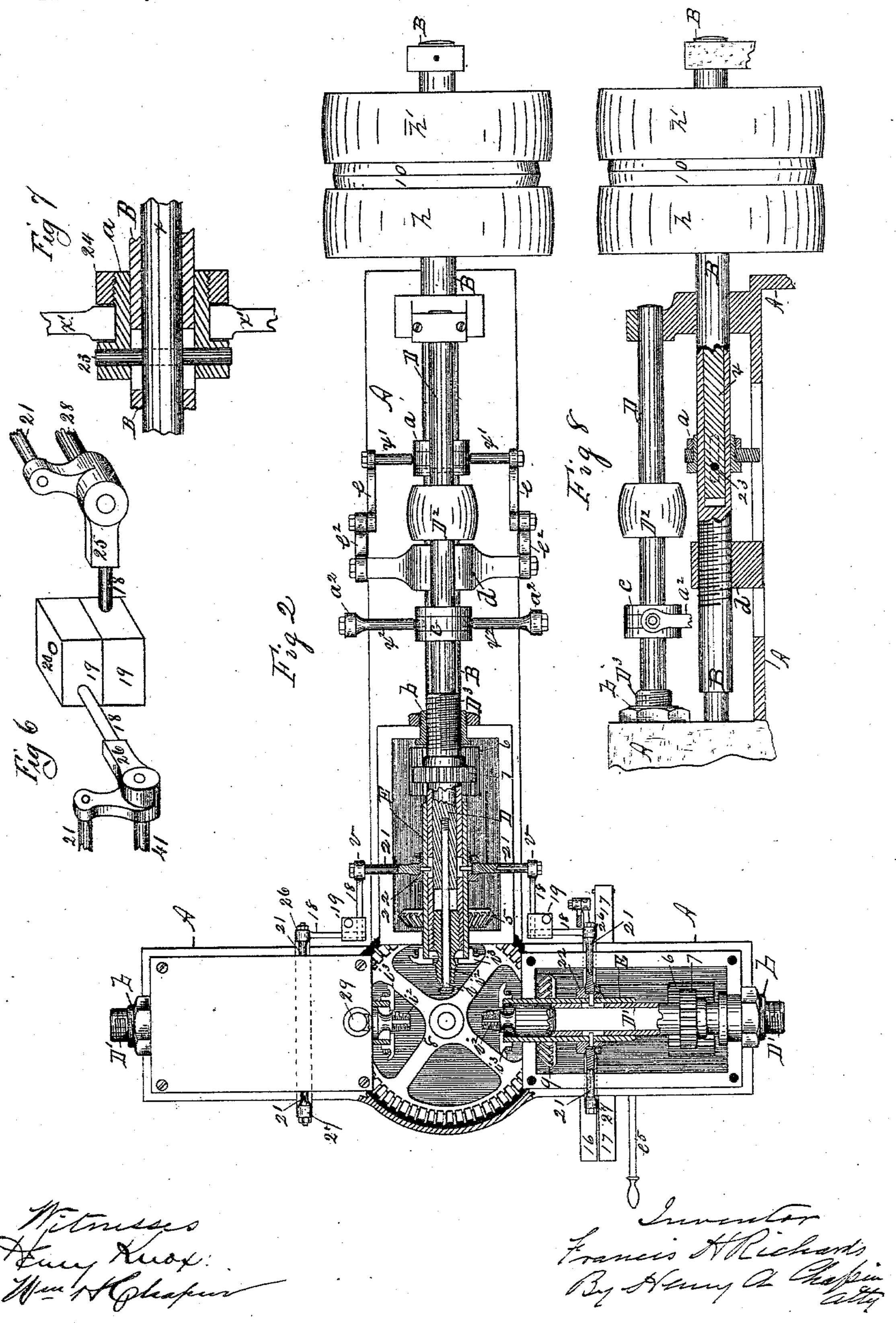
MACHINE FOR FINISHING GLOBE VALVE BODIES.
