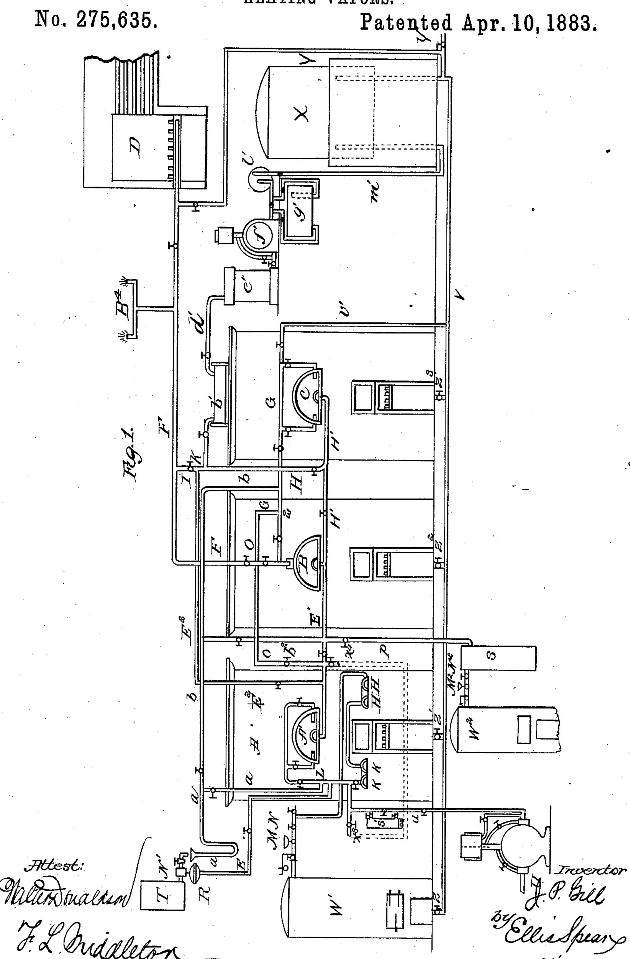
PROCESS OF AND APPARATUS FOR MANUFACTURING LIGHTING OR HEATING VAPORS.
