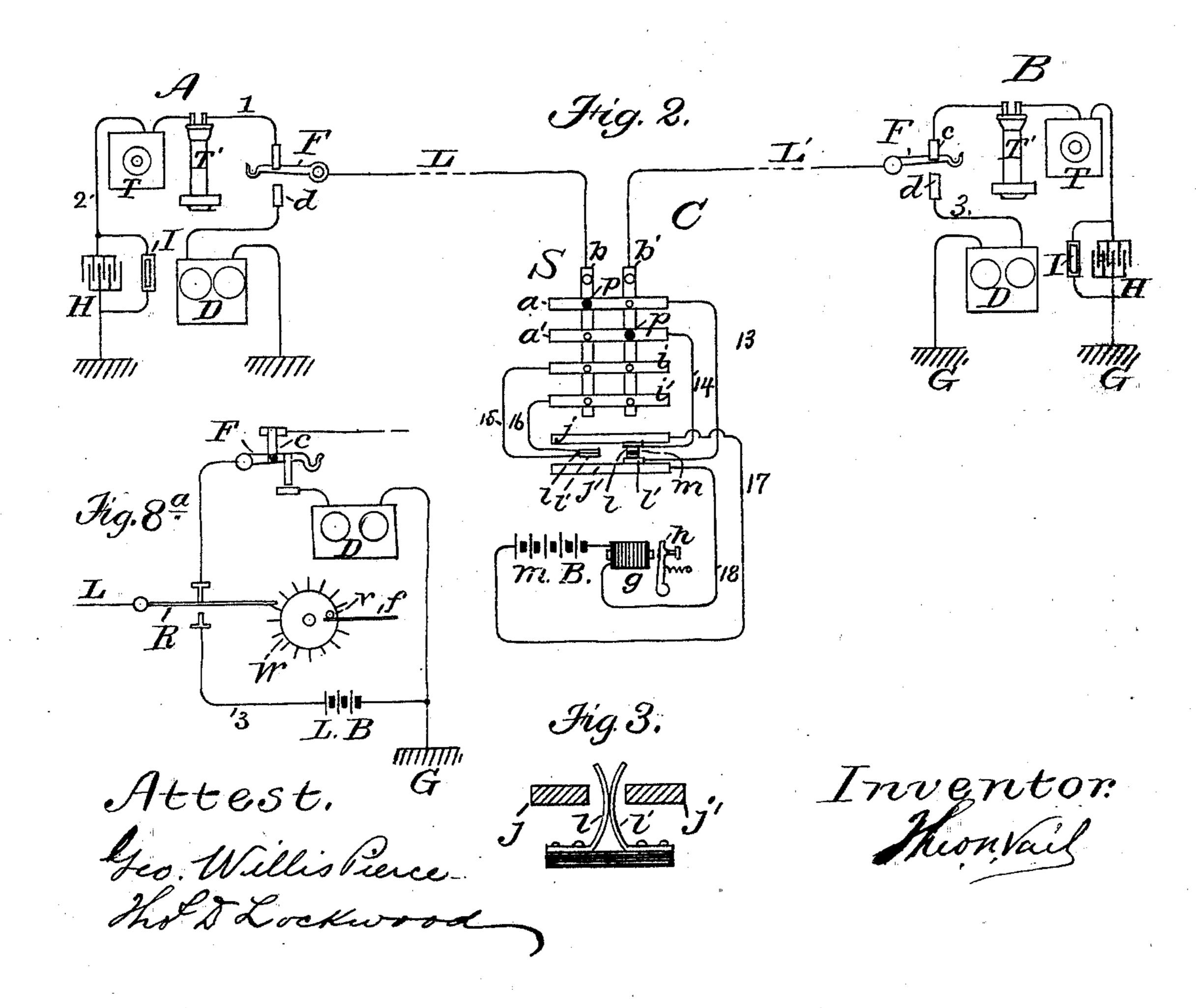
TELEPHONE EXCHANGE SIGNALING CIRCUIT AND APPARATUS. Patented Mar. 27, 1883. No. 274,857. Fig. 8.
