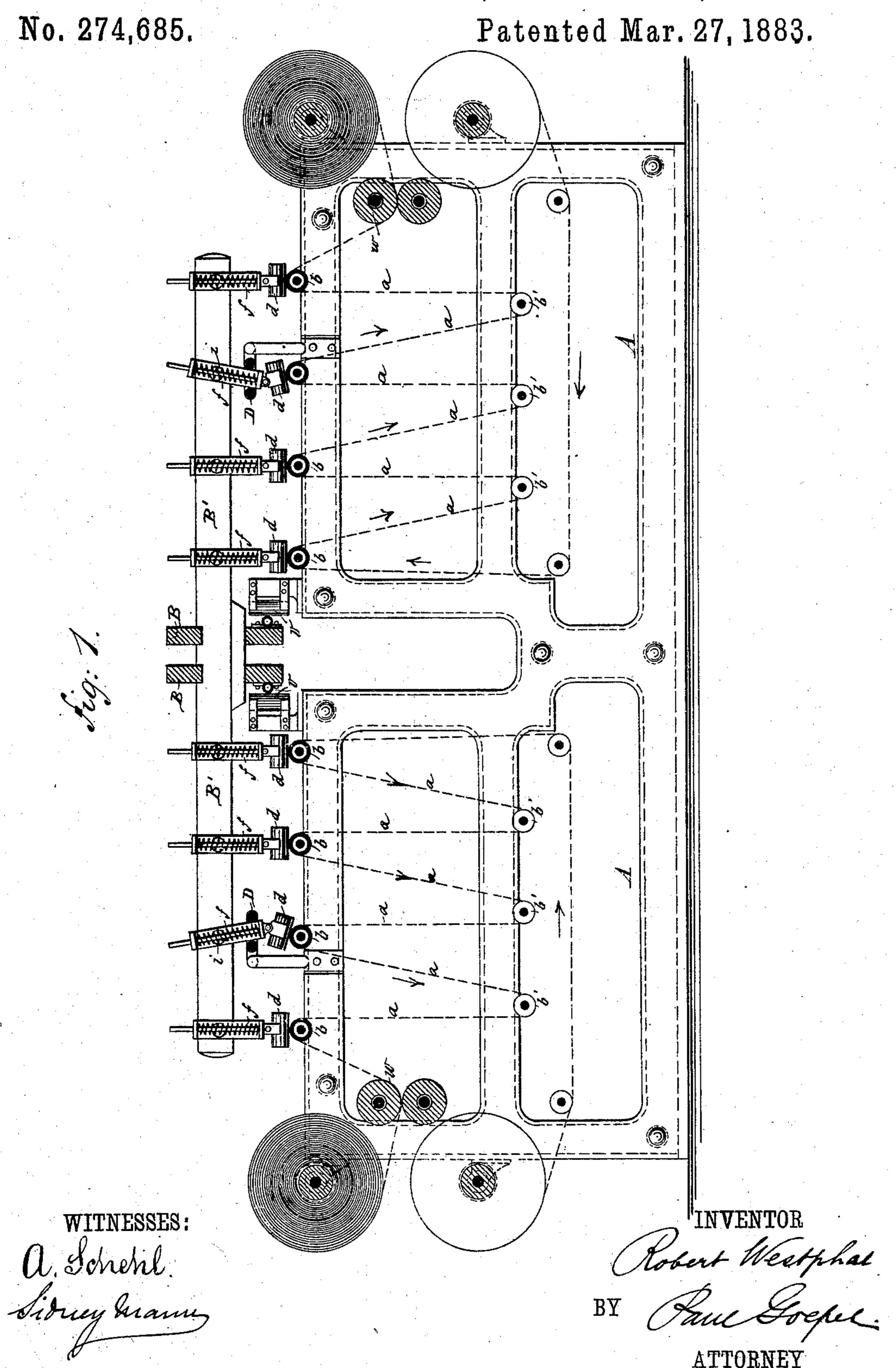
MACHINE FOR POLISHING PAPER, TEXTILE FABRIC, &c.
