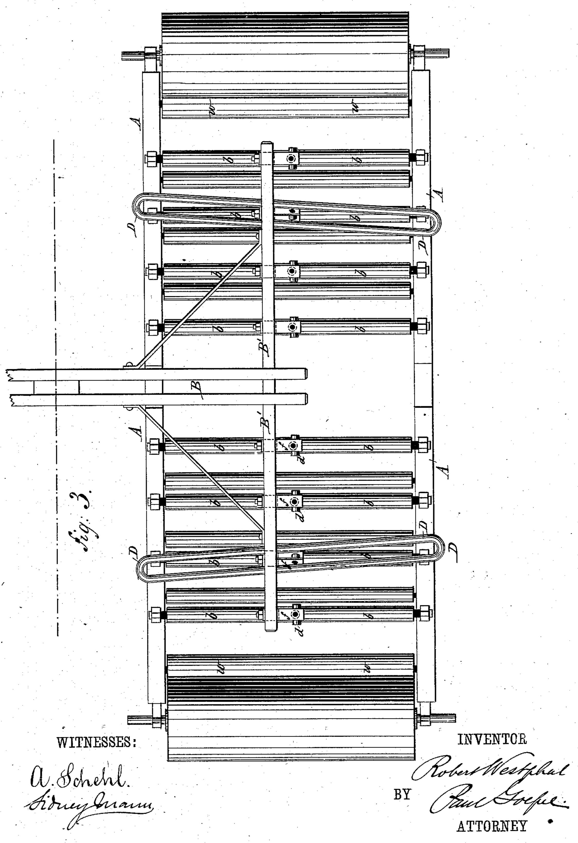
MACHINE FOR POLISHING PAPER, TEXTILE FABRIC, &c.
