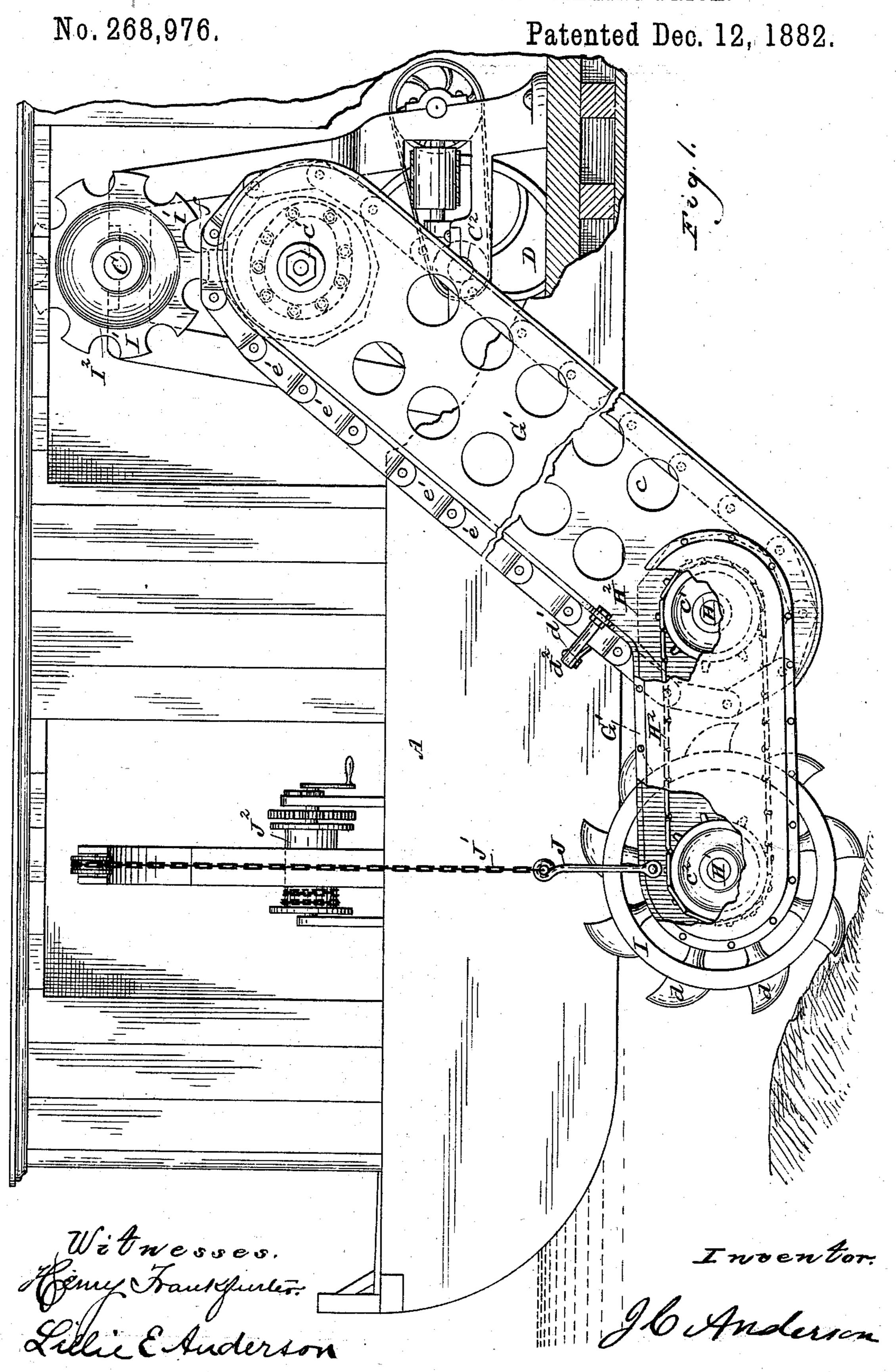
METHOD OF AND APPARATUS FOR MAKING BRICK.
