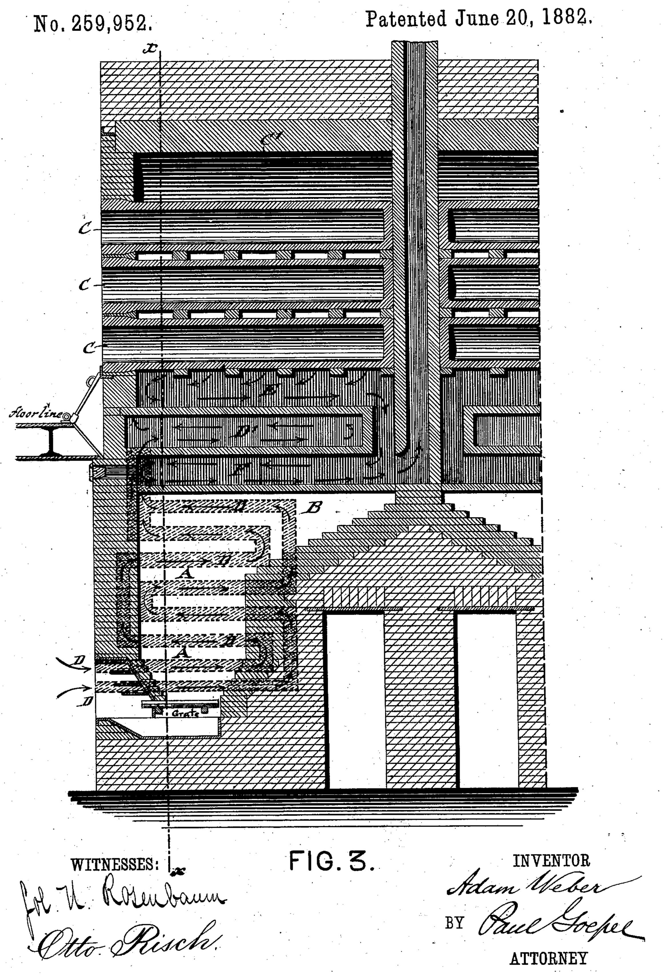
GAS GENERATING FURNACE FOR HEATING RETORTS.
