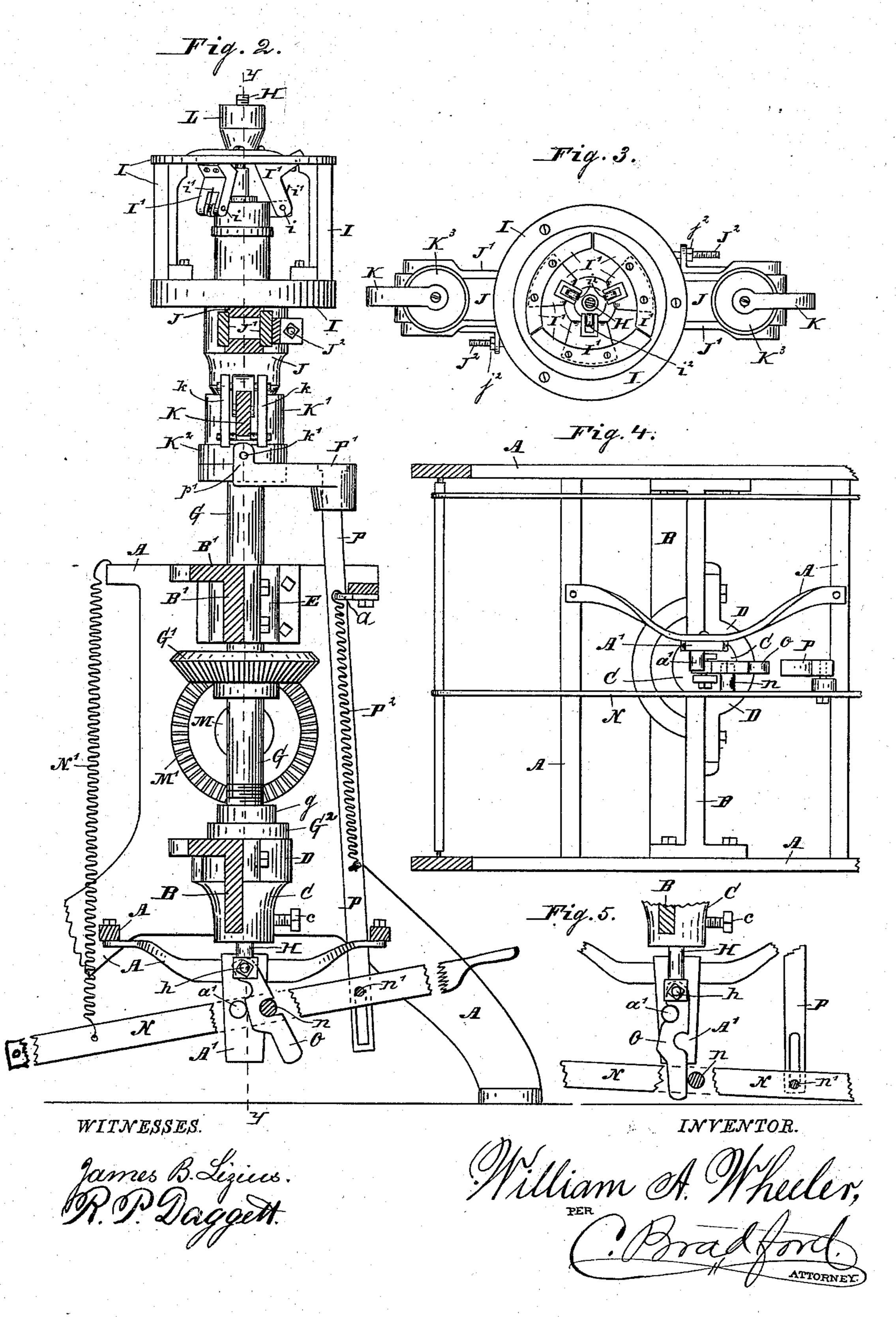
MACHINE FOR CLOSING DOWN THE SEAMS OF SHEET METAL PIPES.
