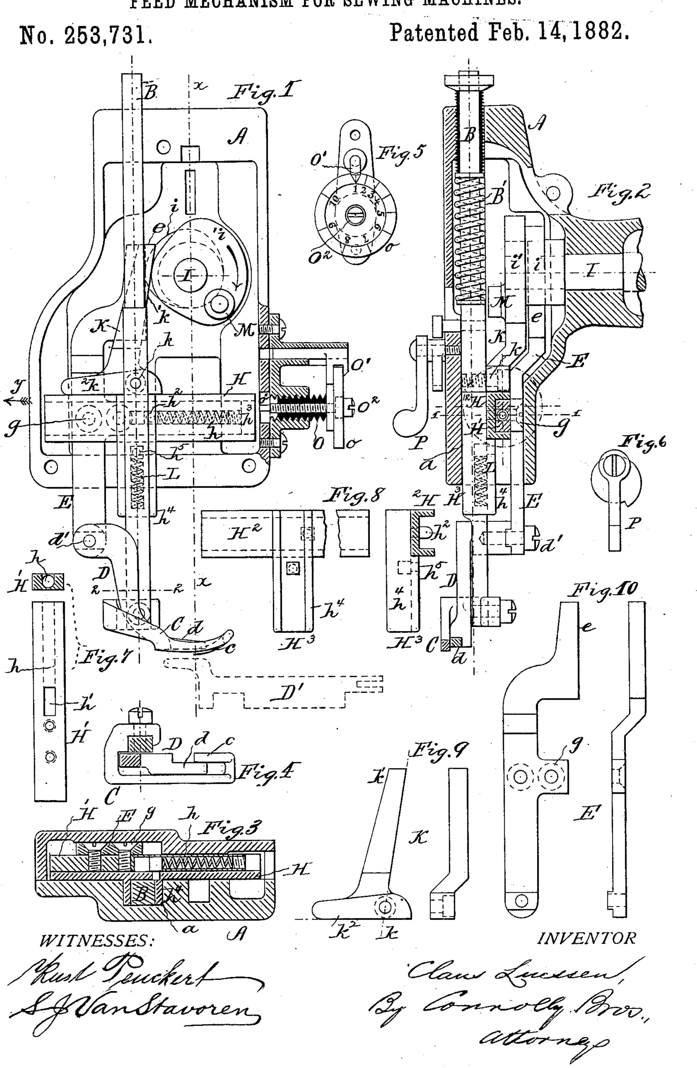
FEED MECHANISM FOR SEWING MACHINES.
