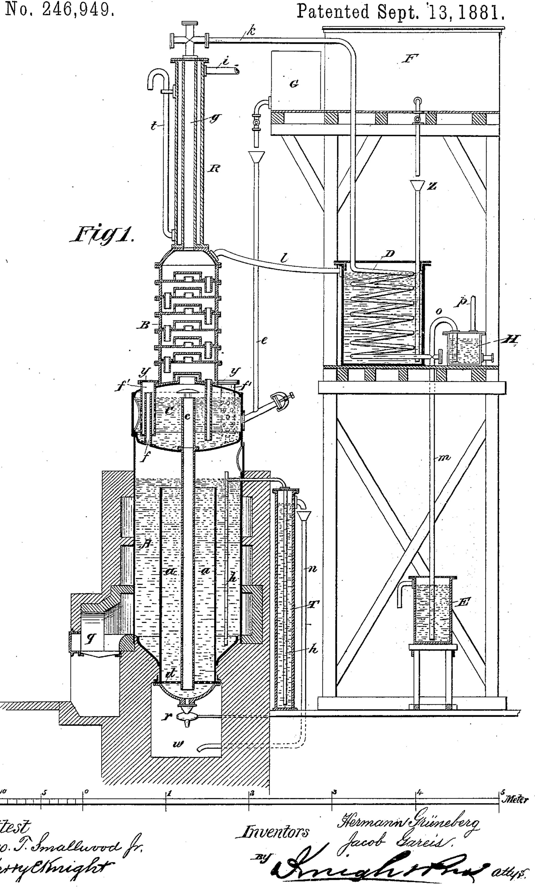
APPARATUS FOR THE CONTINUOUS DISTILLATION OF AMMONIA.
