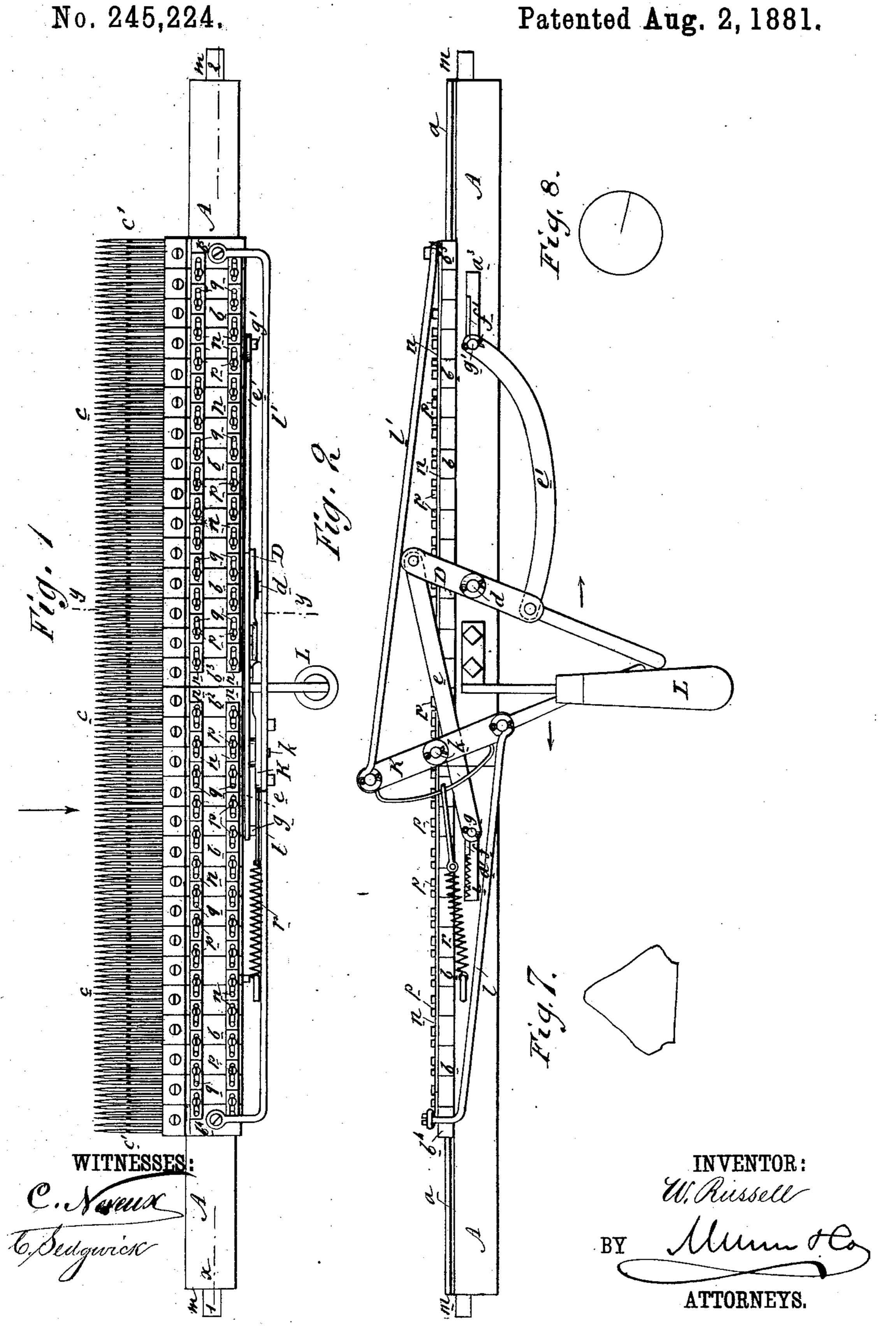
APPARATUS FOR USE IN THE MANUFACTURE OF SCOTCH BONNETS, &c.
