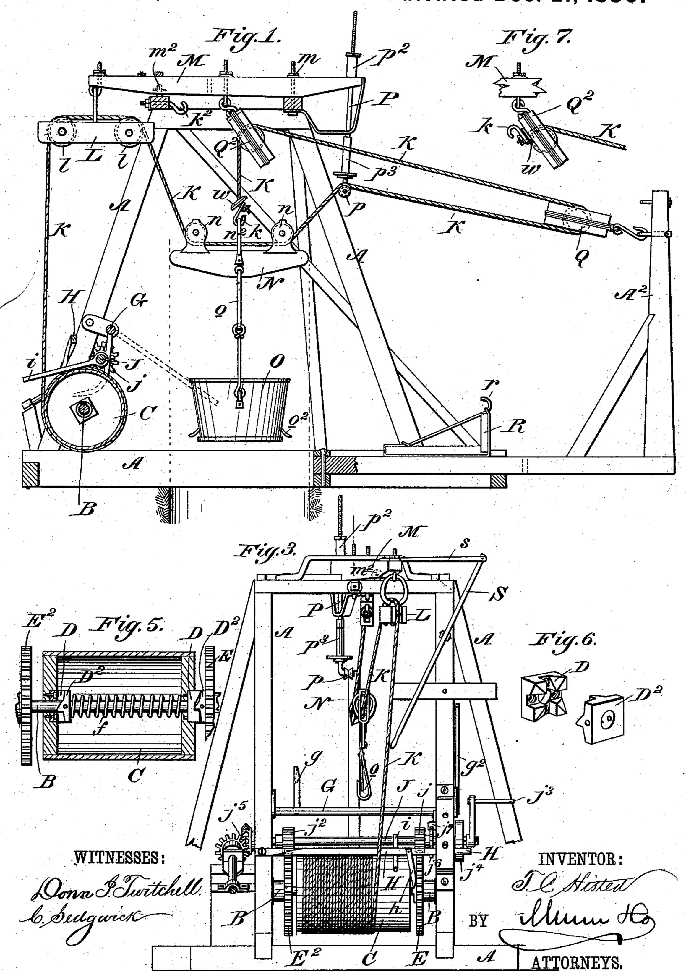
Hoisting Apparatus for Mining Shafts. No. 235,681. Patented Dec. 21.
