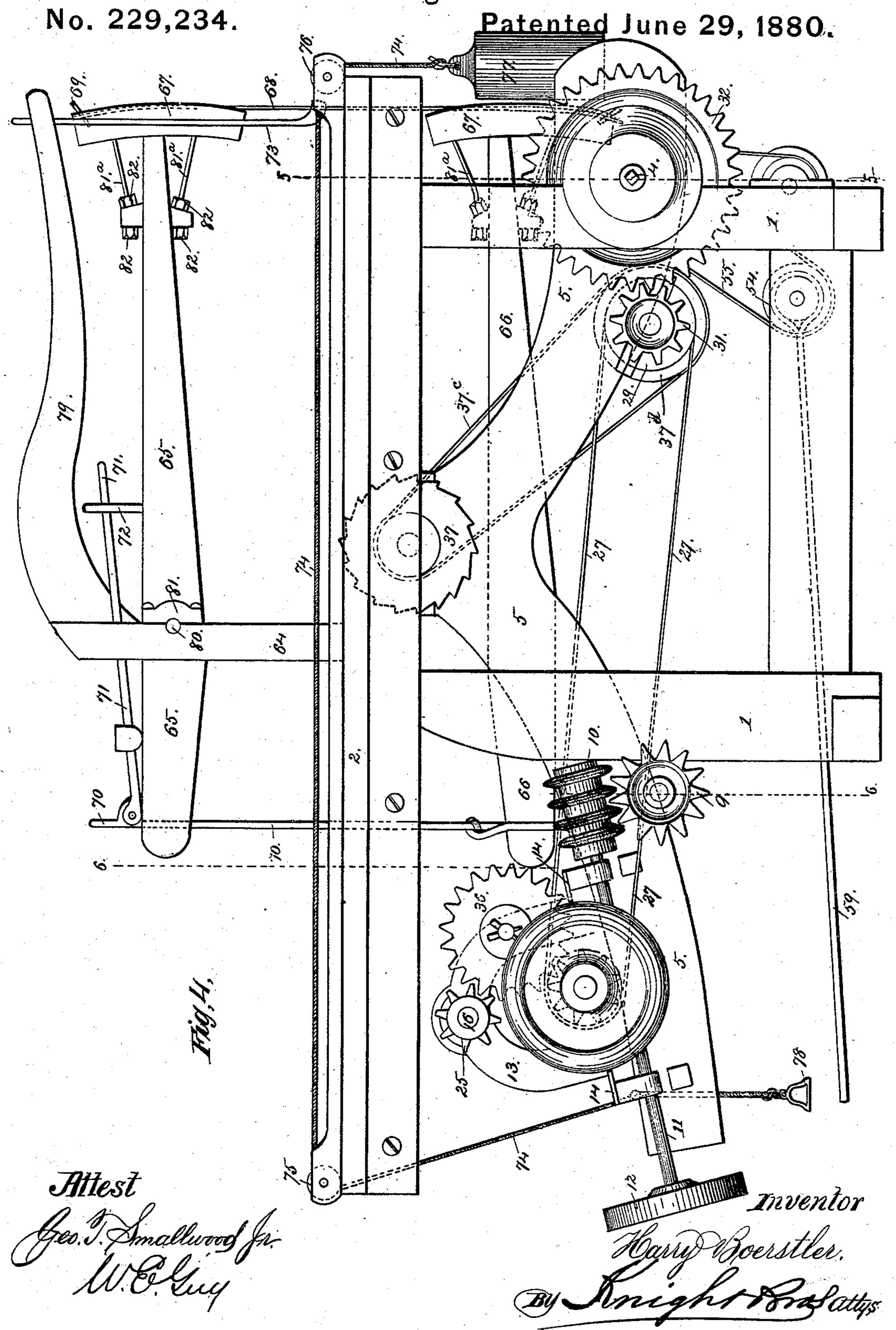
Combined Boring, Sawing, Grinding, and Rabbeting Machine.
