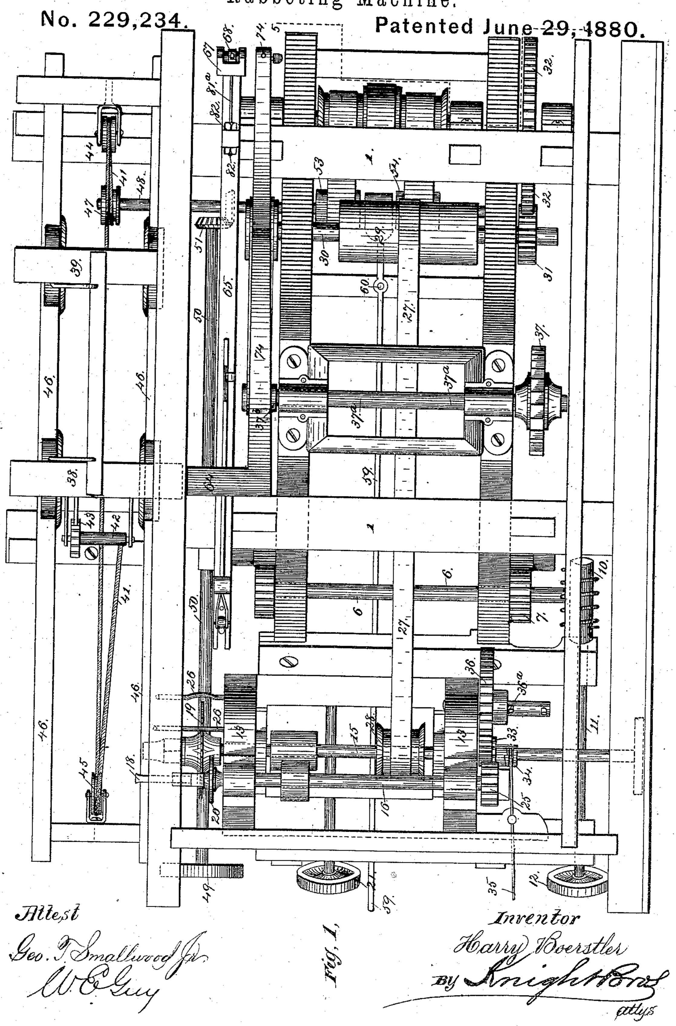
Combined Boring, Sawing, Grinding, and Rabbeting Machine.
