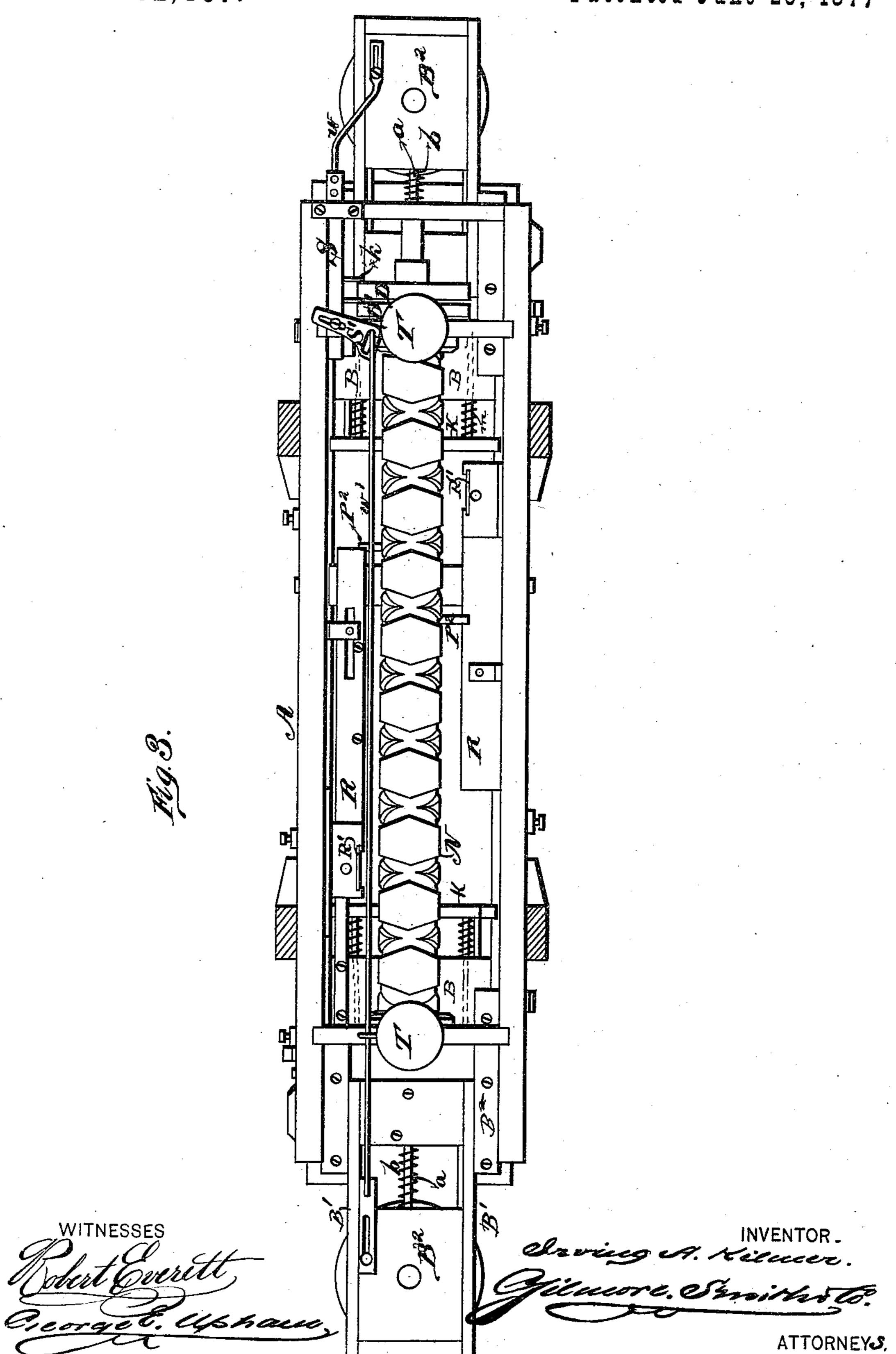
WIRE STRAIGHTENING AND CUTTING MACHINE.
