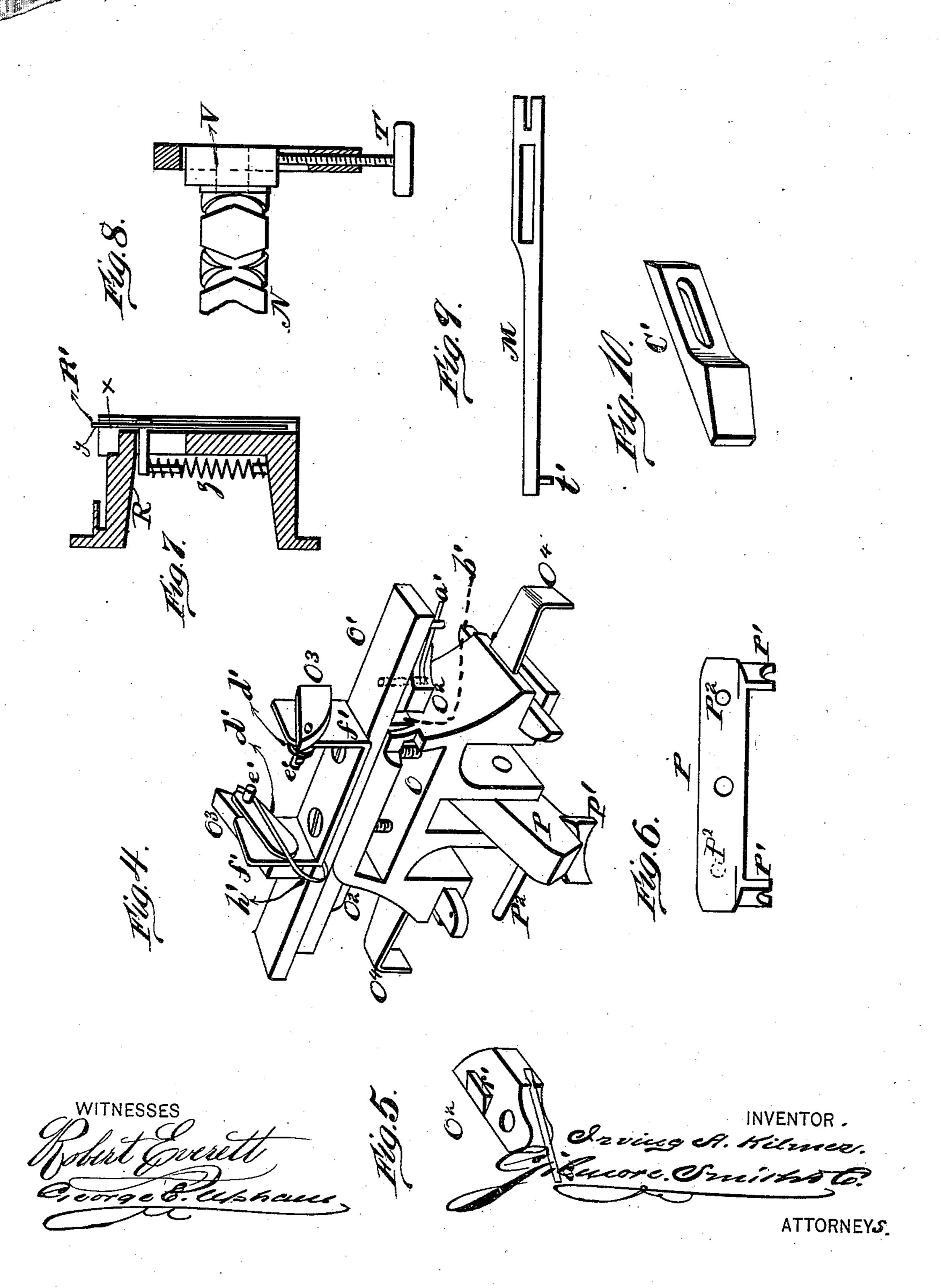
WIRE STRAIGHTENING AND CUTTING MACHINE.
