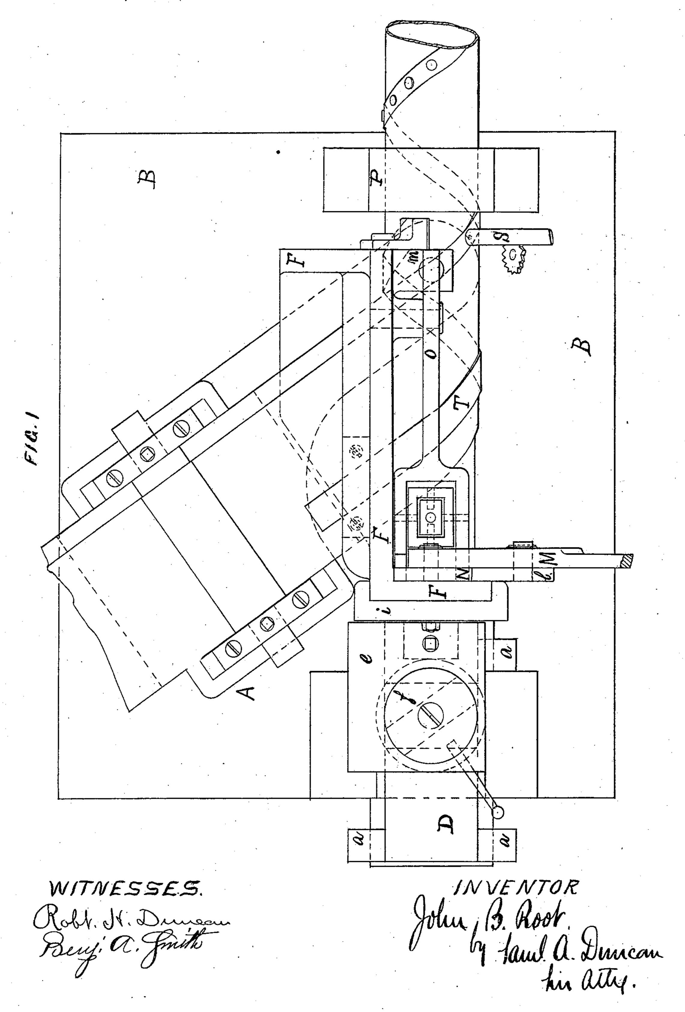
MACHINE FOR MAKING SPIRAL-JOINTED METALLIC TUBING. No. 183,329. Patented Oct. 17, 1876.
