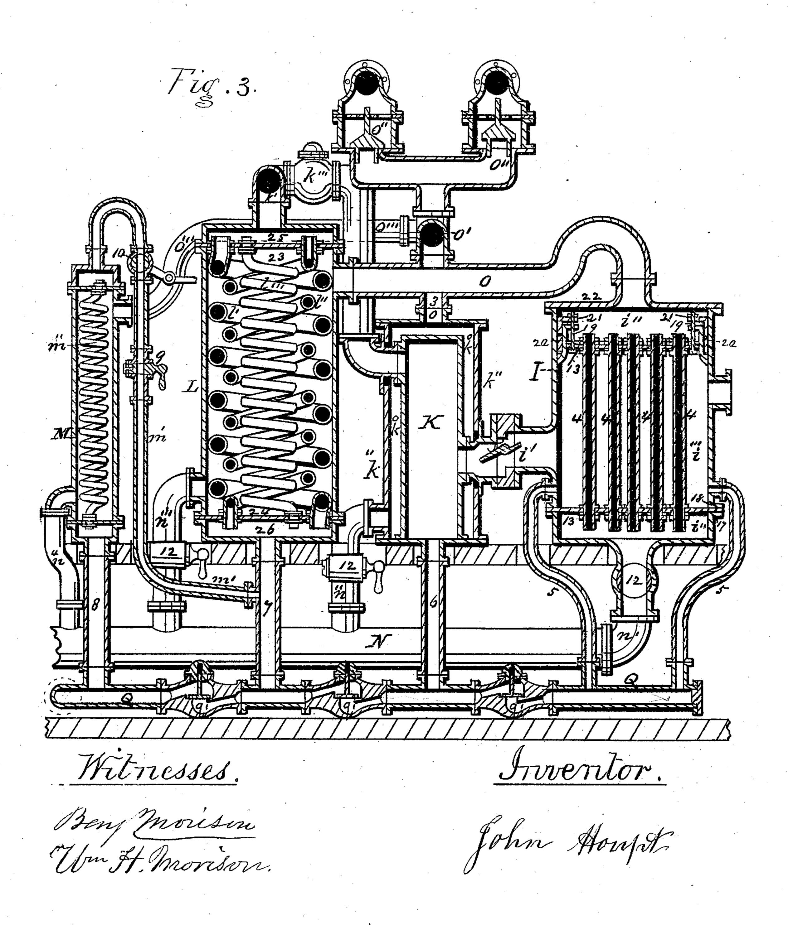
Condensing Apparatus for Marine Steam-Engines.
