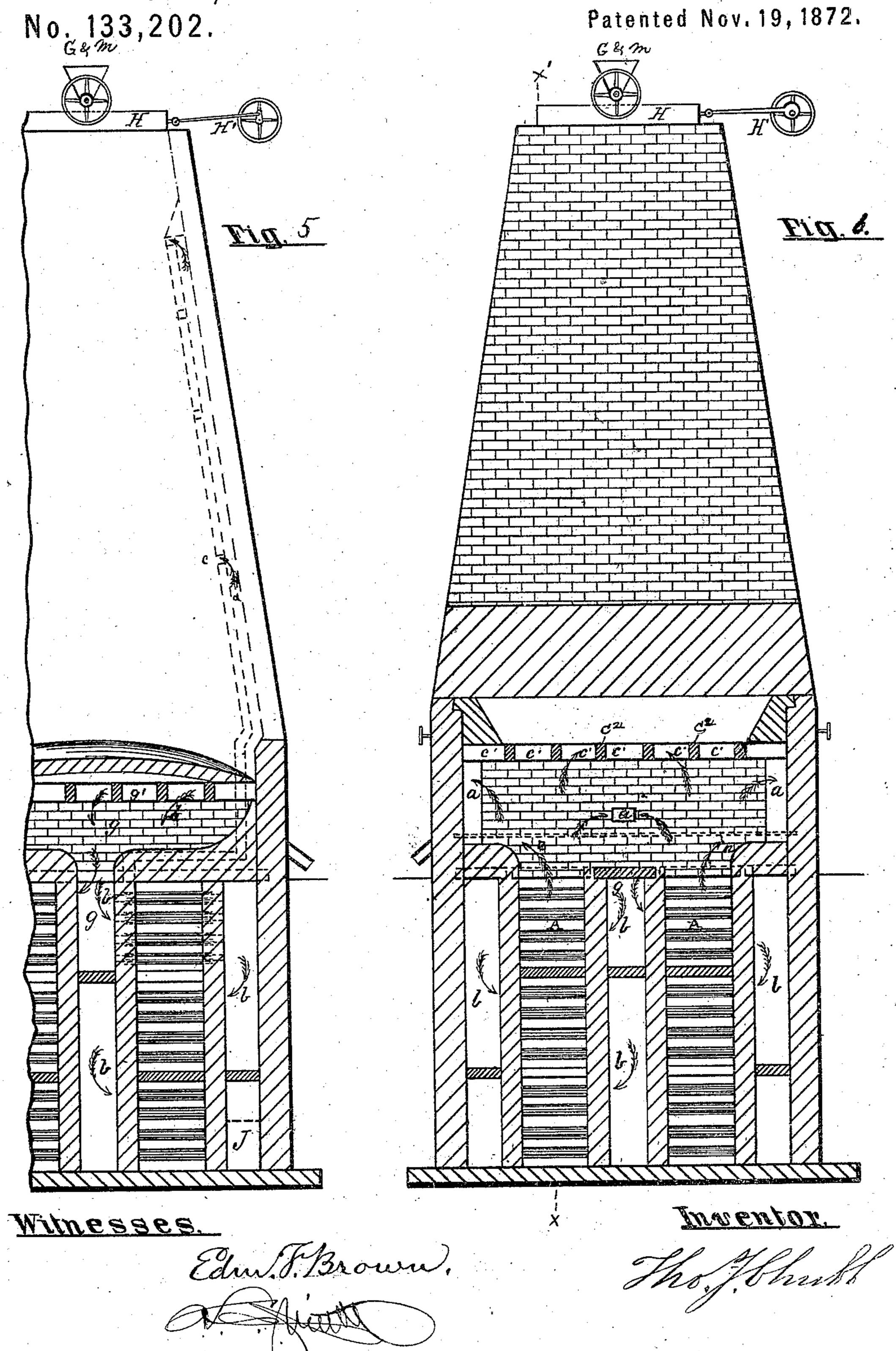
Improvement in Process and Furnace for Making Gas, Iron, and Steel Direct from the Ore.
