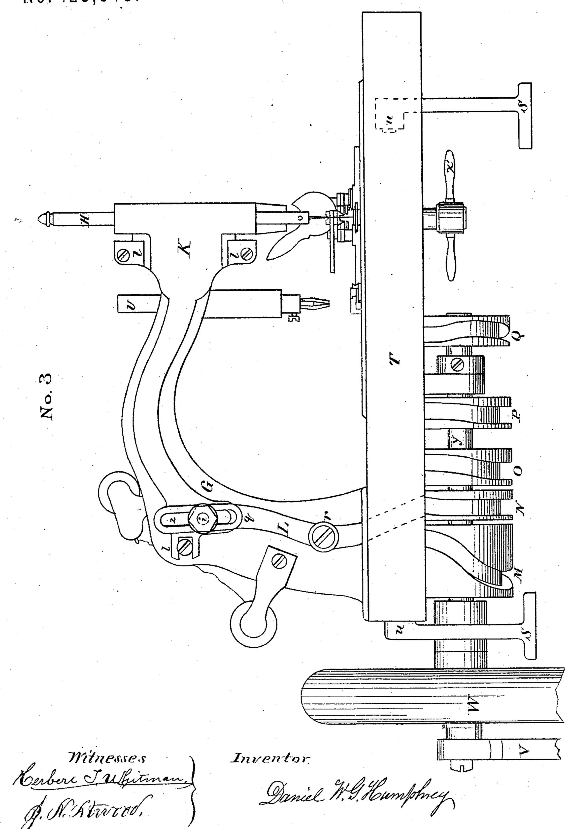
Improvement in Machine for Stitching Button Holes. No. 123,348.
