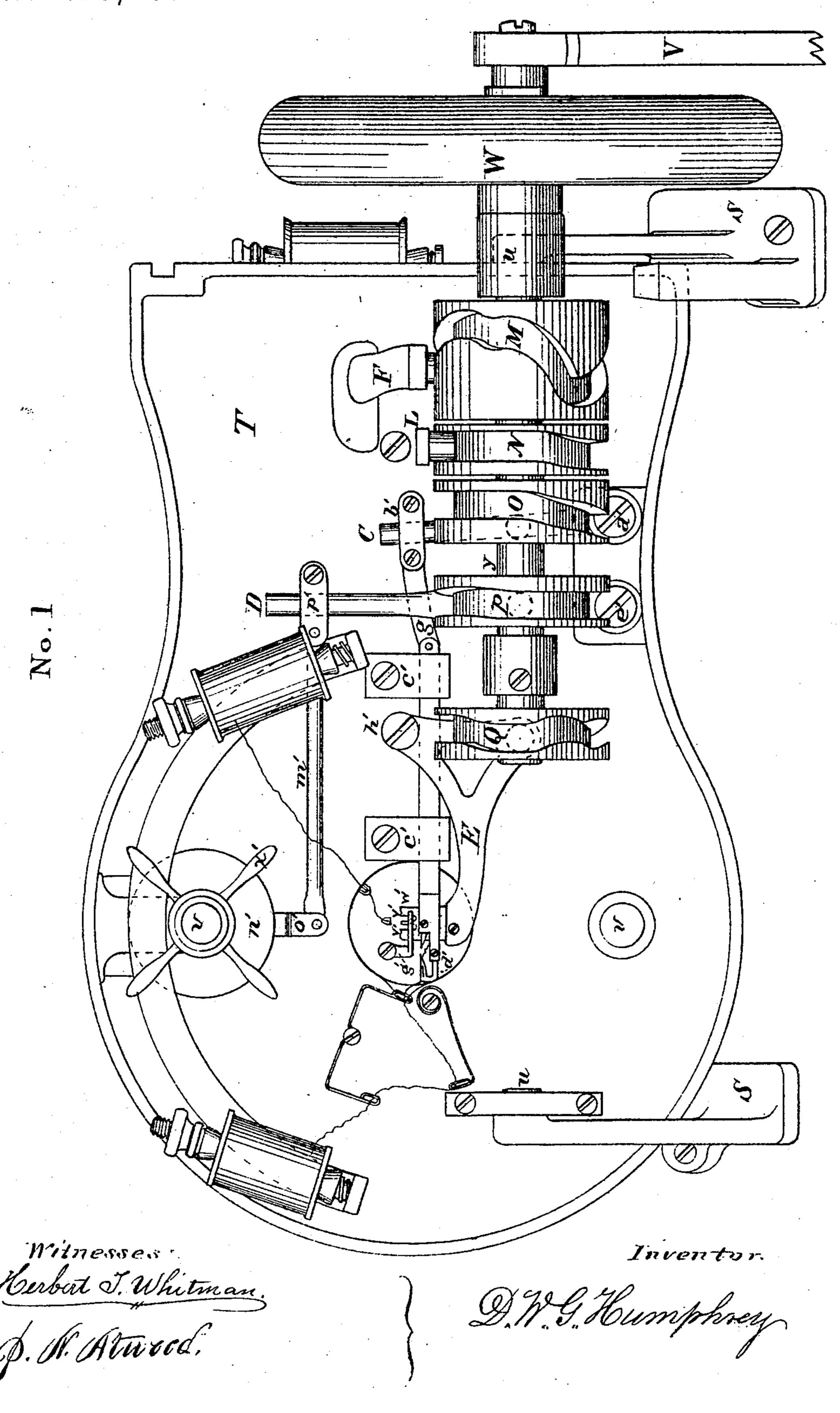
Improvement in Machine for Stitching Button Holes. No. 123,348. Patented Feb. 6, 1872.
